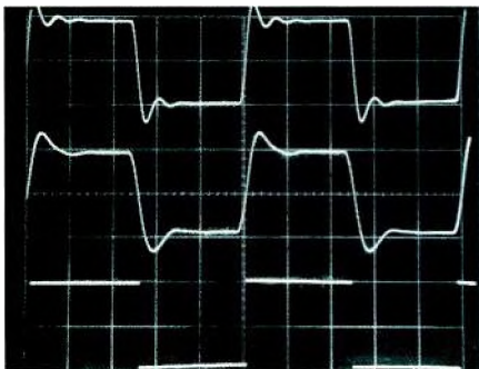
Fig. 2—Square-wave response (from top) at 10 kHz, 8 ohms (20 \mu S/div.); 10 kHz, 8 ohms & 2 \mu F (20 \mu S/div.), and 40 Hz, 8 ohms (5 mS/div.).
