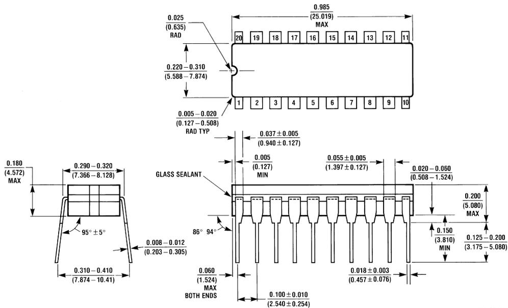
**20 Lead Ceramic Dual-In-Line Package (D)**
