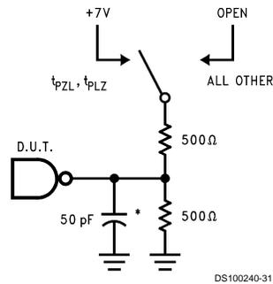
\*Includes jig and probe capacitance
