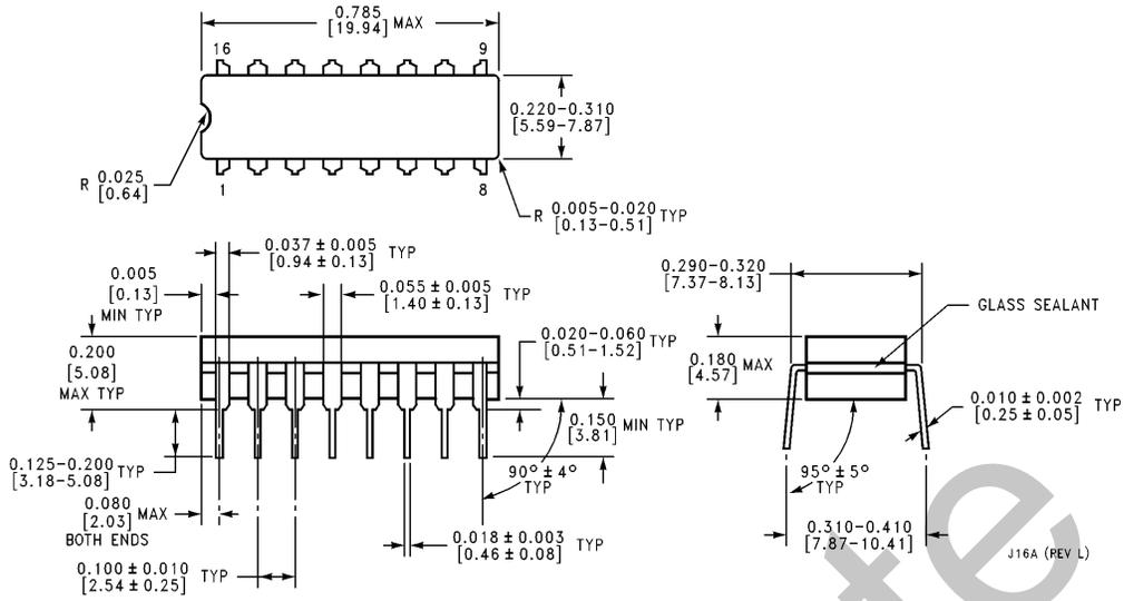
**16-Lead Ceramic Dual-In-Line Package (D)
