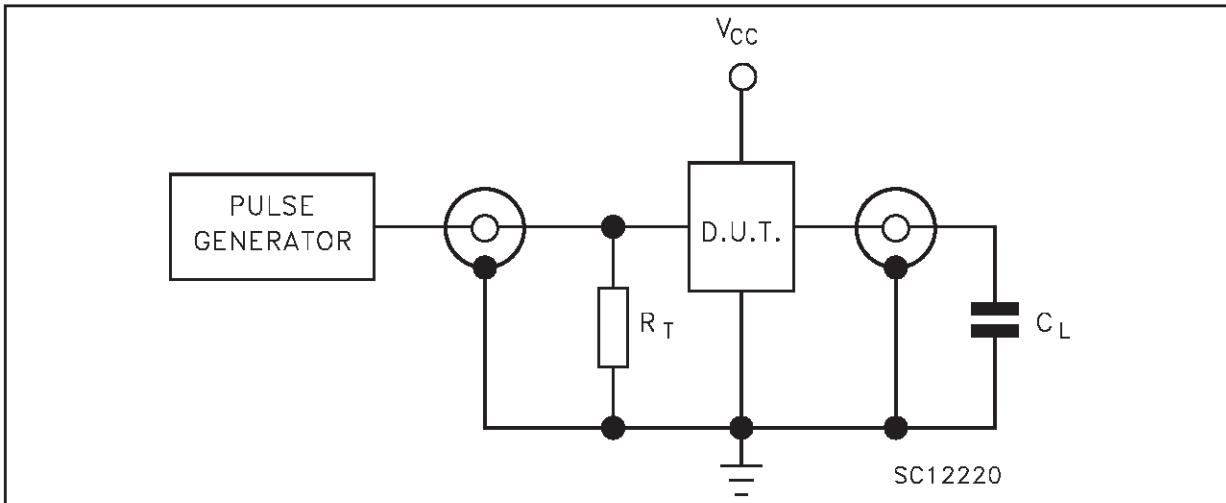
$C_L = 15/50 \mu\text{F}$  or equivalent (includes jig and probe capacitance) $R_T = Z_{OUT}$  of pulse generator (typically  $50\Omega$ )
