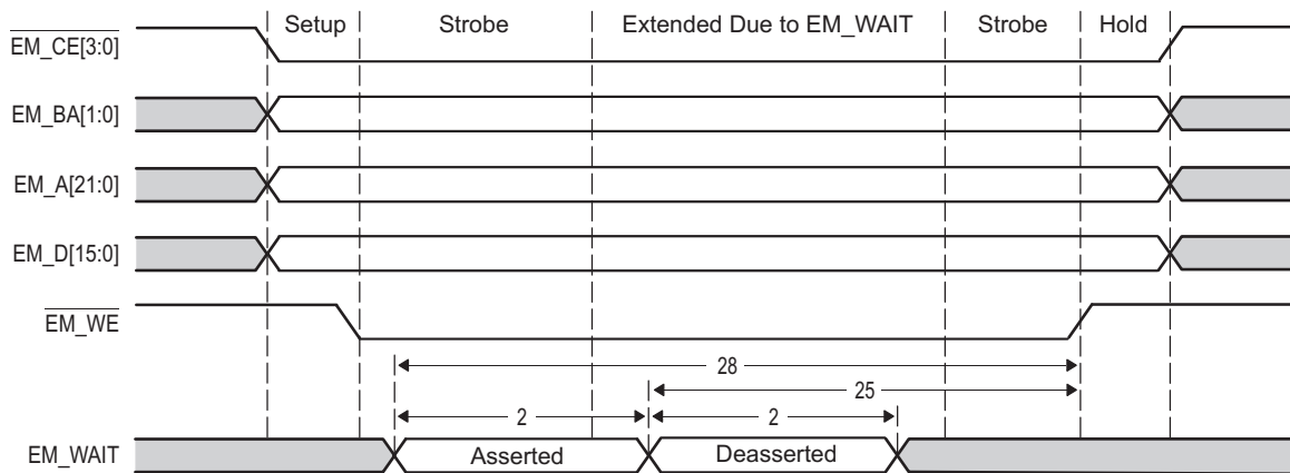
Figure 9-54 EMIF16 EM_WAIT Write Timing Diagram
