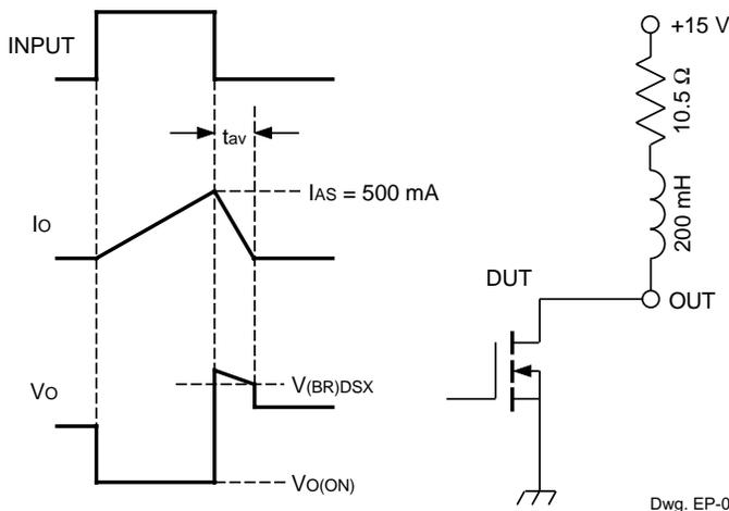
**Single-Pulse Avalanche Energy Test Circuit
