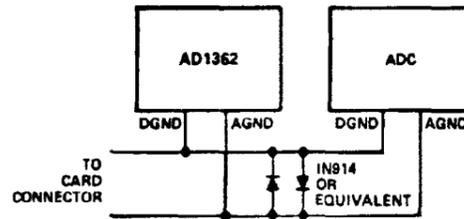
Figure 4. Ground-Fault Protection Diodes
