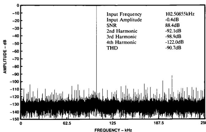
Figure 21. Full-Scale Power Spectral Density at  $T_{CASE} = +125^{\circ}\text{C}$ , Calibration Performed at  $T_{CASE} = +25^{\circ}\text{C}$ ,  $\pm 5\text{ V}$  Range, 16384-Point FFT, 500 kHz Sample Rate
