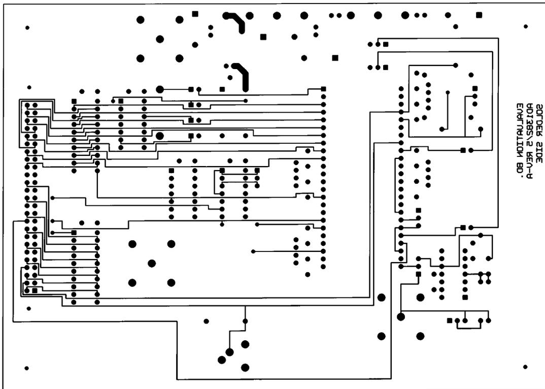
Figure 33. AD1385 Evaluation Board Layout, Layer 4 (Solder Side)
