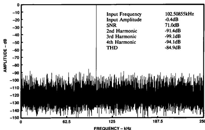
Figure 20. Full-Scale Power Spectral Density after Power-up at  $T_{CASE} = +25^{\circ}\text{C}$  Without Calibration,  $\pm 5\text{ V}$  Range, 16384-Point FFT, 500 kHz Sample Rate. Compare with Figure 4.
