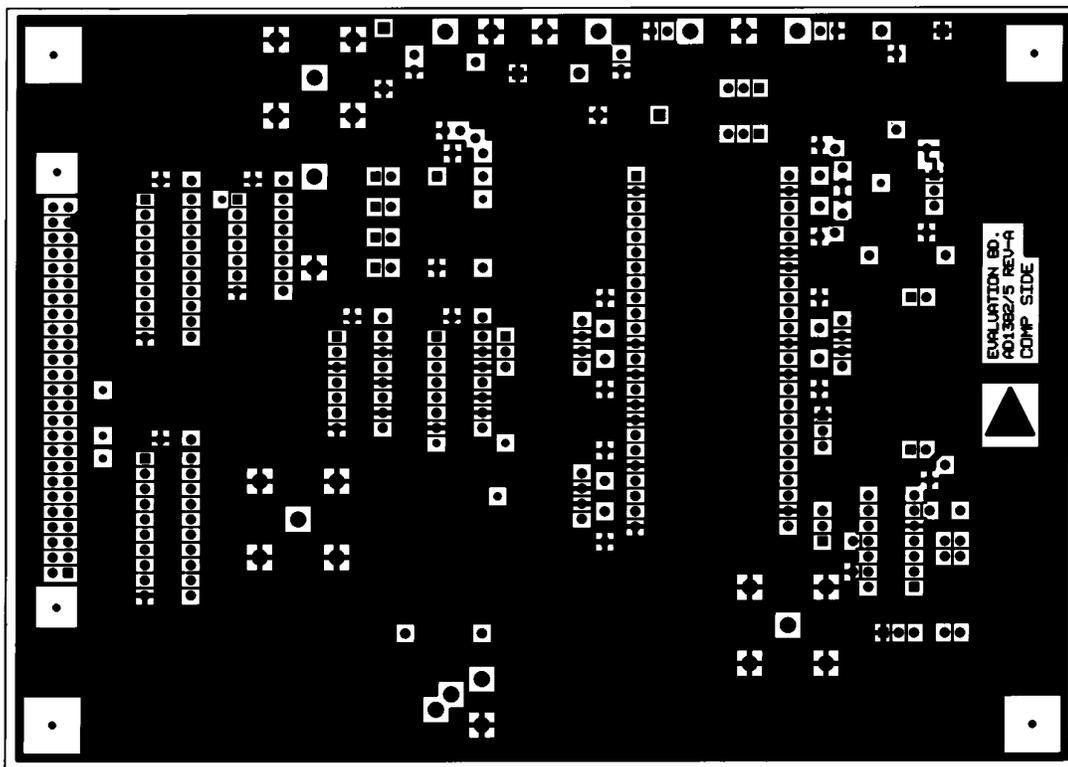
Figure 30. AD1385 Evaluation Board Layout, Layer 1 (Component Side)
