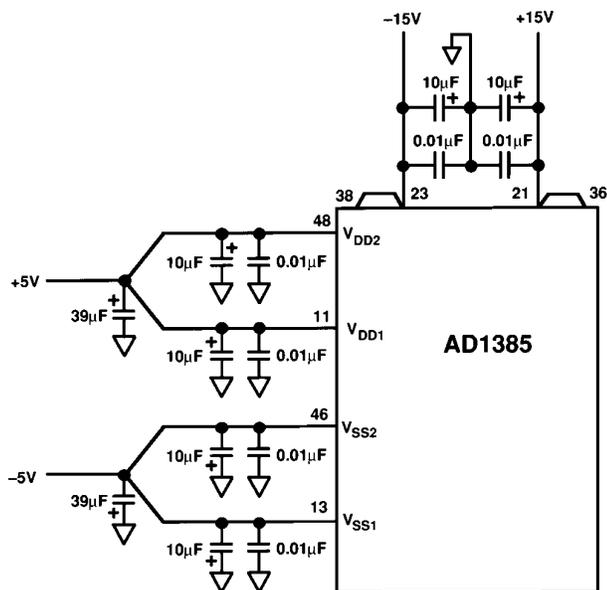
Figure 15. Recommended AD1385 Power Distribution. All 10  $\mu\text{F}$  and 0.01  $\mu\text{F}$  capacitors must have minimum lead length and be located as close as possible to the bypassed pins. Make all ground connections directly to the ground plane.
