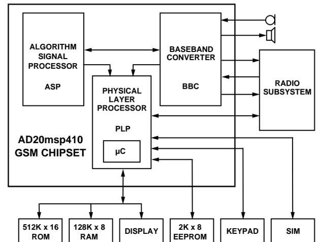
preprogrammed ROM, no user programming is required. The ASP implements full rate speech transcoding according to GSM specifications, including Discontinuous Transmission (DTX) and Comfort Noise Insertion (CNI). A high performance soft-decision Viterbi equalizer is also implemented in software, embedded in the ROM.
