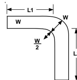
Figure 7. PCB Track Shunt Resistor with  $90^\circ$  Bend
