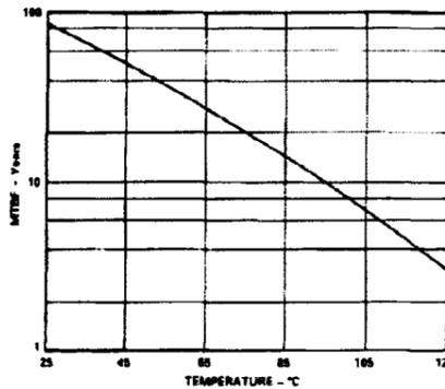
Figure 6. 2S44 MTBF vs. Temperature
