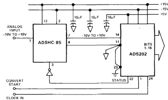
Figure 8. 18.3kHz-12-Bit, A/D Conversion System
