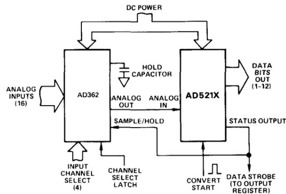
Figure 10. High Speed 12-Bit DAS
