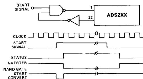
Figure 11. Convert Start Using a Positive Edge
