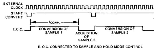
Figure 9. START/E.O.C. Timing for Sampled Data System
