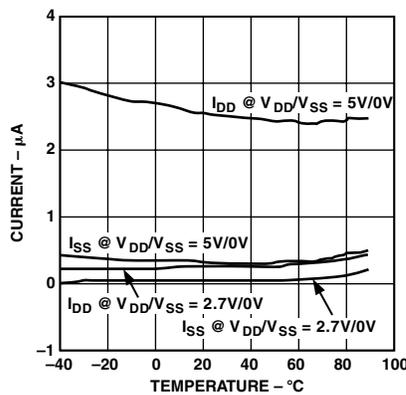
TPC 8.  $I_{DD}$  vs. Temperature,  $R_{AB} = 10\text{ k}\Omega$
