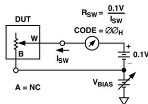
Test Circuit 8. Incremental ON Resistance
