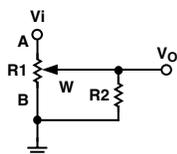
Figure 28. Resistor Scaling with Pseudo Log Adjustment Characteristics
