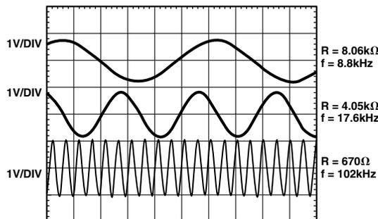
Figure 22. Programmable Oscillation
