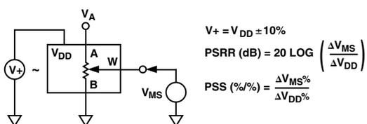
Test Circuit 4. Power Supply Sensitivity (PSS, PSRR)
