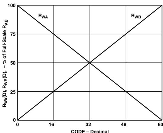
Figure 10.  $R_{WA}(D)$  and  $R_{WB}(D)$  vs. Decimal Code
