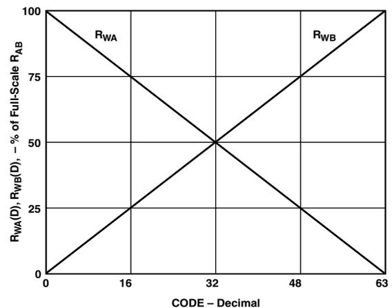
Figure 1.  $R_{WA}(D)$  and  $R_{WB}(D)$  vs. Decimal Code
