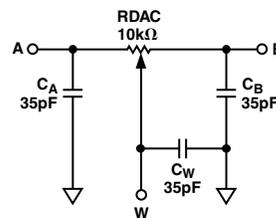
Figure 32. RDAC Circuit Simulation Model for RDAC = 10 kΩ
