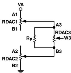
Figure 29. Doubling AD5233 from 6-Bit to 12-Bit
