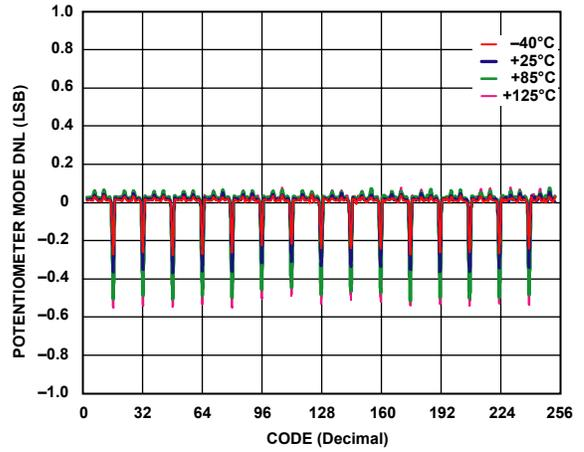
Figure 6. DNL vs. Code,  $V_{DD} = 5 V$
