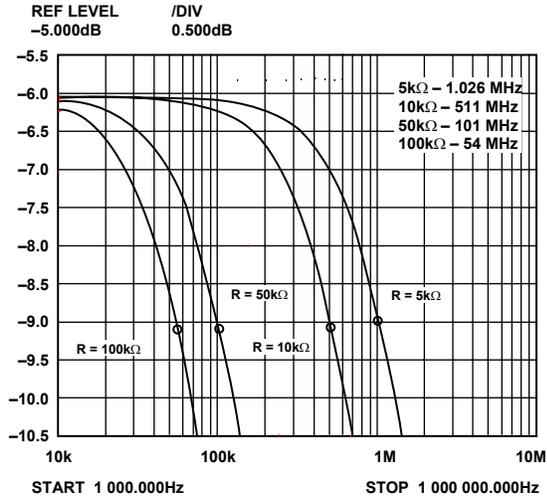
Figure 21. -3 dB Bandwidth @ Code = 0x80
