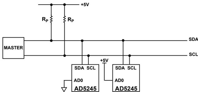
Figure 40. Multiple AD5245 Devices on One I<sup>2</sup>C Bus
