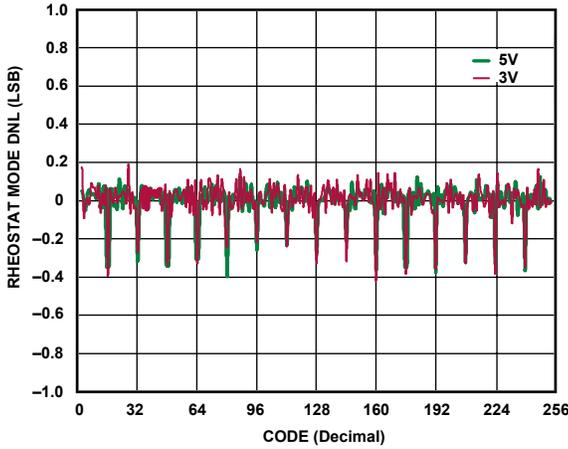
Figure 4. R-DNL vs. Code vs. Supply Voltages
