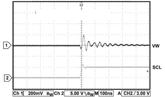
Figure 24. Digital Feedthrough
