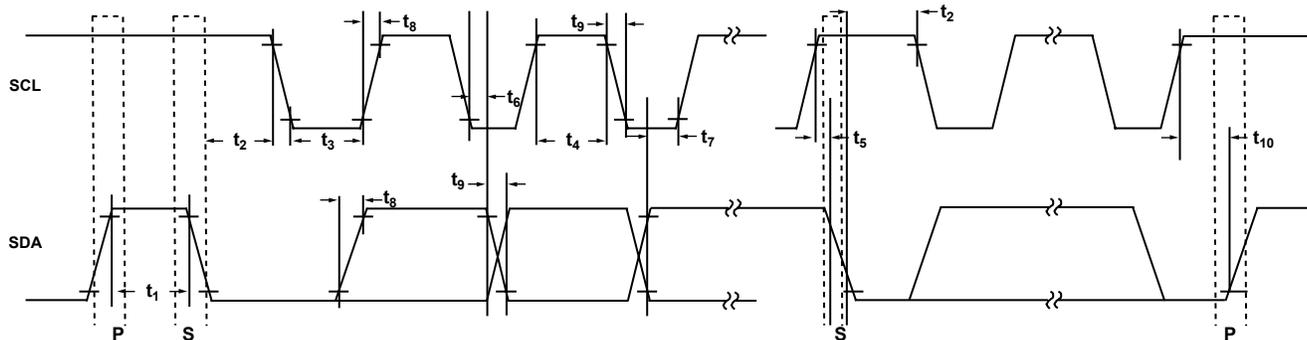
Figure 36. I<sup>2</sup>C Interface Detailed Timing Diagram
