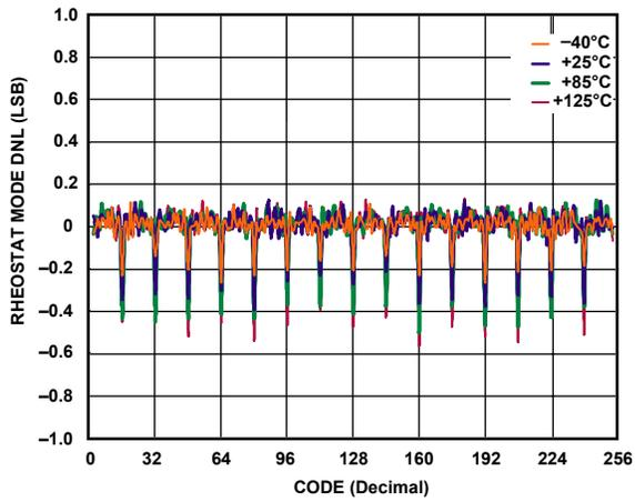
Figure 10. R-DNL vs. Code,  $V_{DD} = 5\text{ V}$
