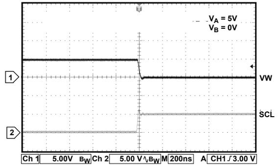
Figure 26. Large Signal Settling Time, Code 0xFF-0x00
