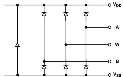
Figure 44. Maximum Terminal Voltages Set by V<sub>DD</sub> and V<sub>SS</sub>
