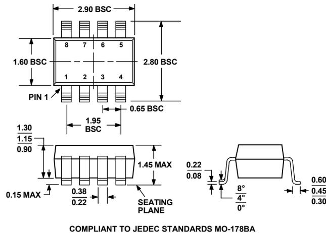
Figure 47. 8-Lead Small Outline Transistor Package [SOT-23] (RJ-8)
