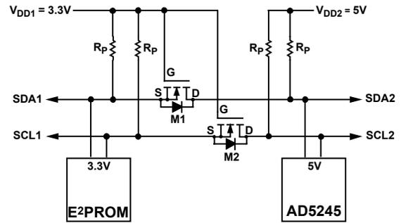
Figure 41. Level Shifting for Operation at Different Potentials
