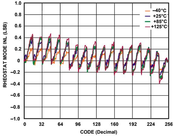
Figure 9. R-INL vs. Code,  $V_{DD} = 5\text{ V}$
