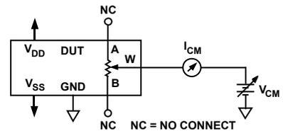
Figure 35. Test Circuit for Common-Mode Leakage current
