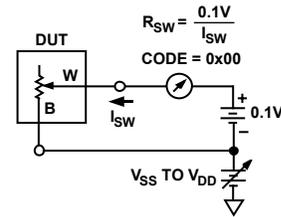
Figure 34. Test Circuit for Incremental ON Resistance
