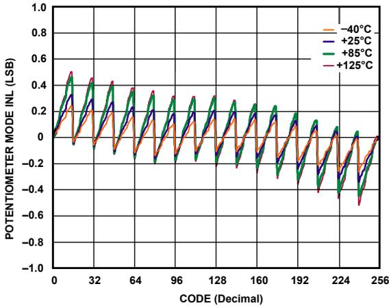
Figure 5. INL vs. Code,  $V_{DD} = 5 V$
