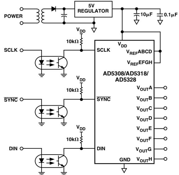
Figure 17. AD5308/AD5318/AD5328 in an Opto-Isolated Interface
