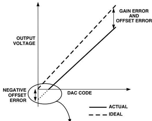
Figure 2. Transfer Function with Negative Offset ( $V_{REF} = V_{DD}$ )
