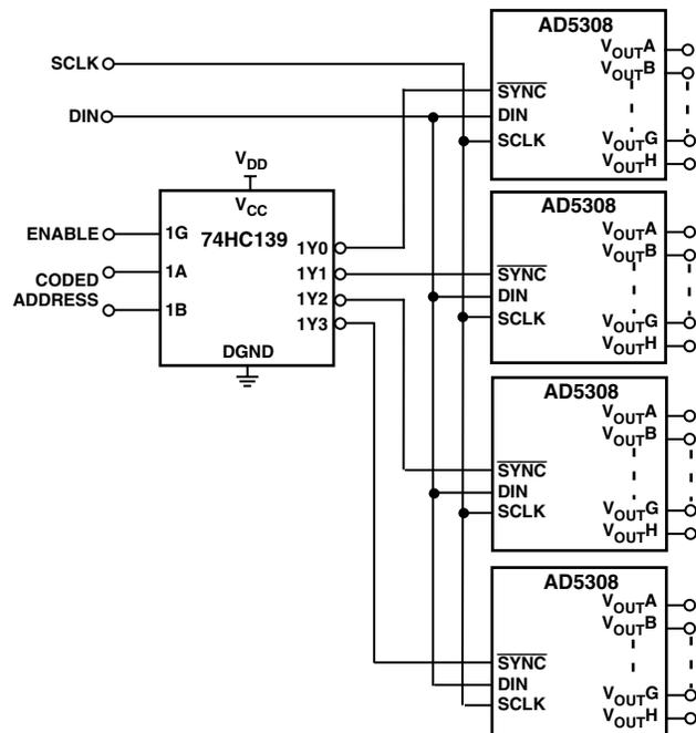
Figure 18. Decoding Multiple AD5308 Devices in a System
