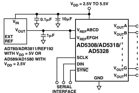
Figure 15. AD5308/AD5318/AD5328 Using a 2.5 V External Reference
