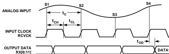
*Figure 5. Receive Interface Timing Diagram*
