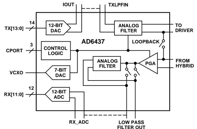
The AD6437 includes both transmit and receive paths. These include the DAC (up to 20 MSPS, allowing for oversampling of the downstream transmit signal), ADC (up to 10 MSPS), low noise PGA and filters. The filters are software configurable for both the CO and RT modes. There is an auxiliary 7-bit auxiliary DAC (e.g., for timing recovery).
