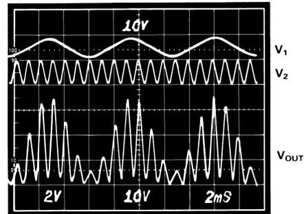
Figure 19. Multiplier Waveforms
