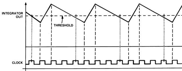
Figure 3. Integrator Output for  $I_{IN} = 250 \mu A$
