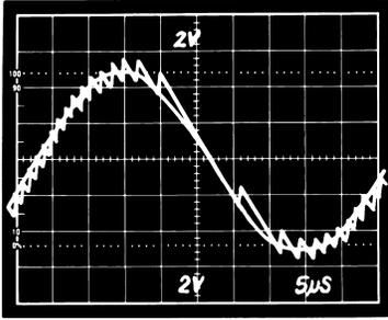
Figure 30. Delta Modulator Input Signal and Ramp-Wise Approximation
