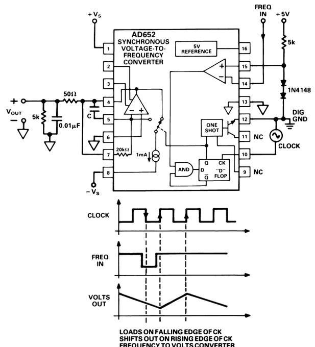
Figure 17. Frequency-to-Voltage Converter
