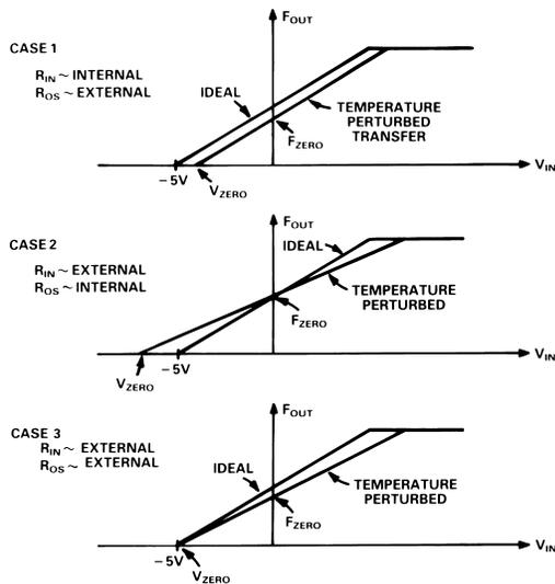
Figure 8c. Actual Bipolar Input Transfer Over Temperature
