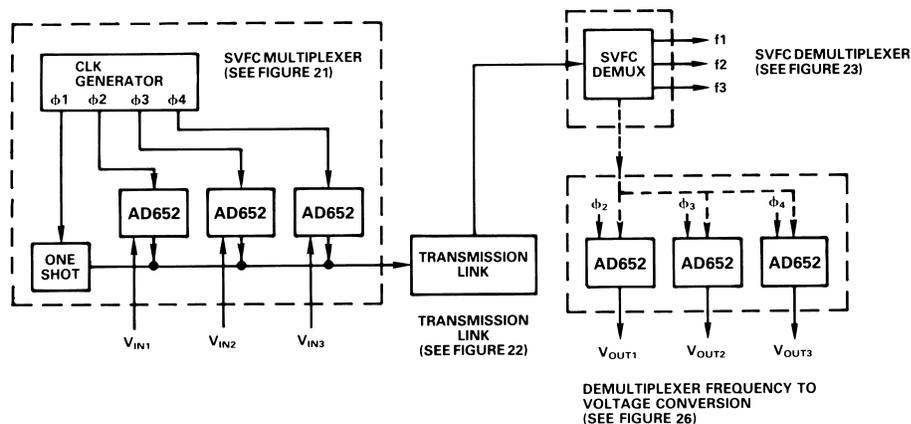
Figure 20. Single Line Multiplexed Data Transmission Block Diagram
