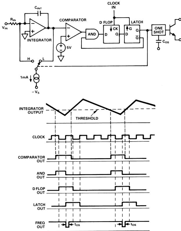
Figure 2. AD652 Block Diagram and System Waveforms
