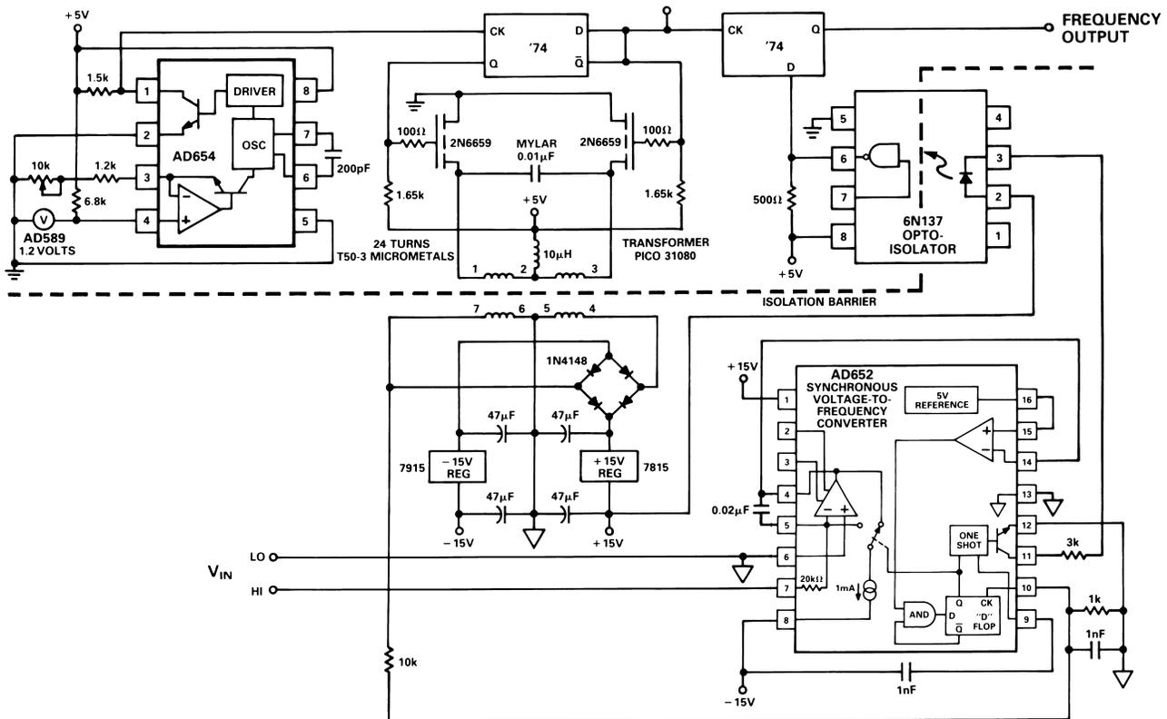
Figure 27. Isolated Synchronous VFC
