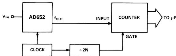
Figure 28. Block Diagram of SVFC A-to-D Converter
