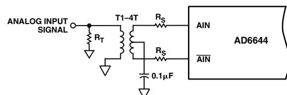
Figure 10. Transformer-Coupled Analog Input Circuit
