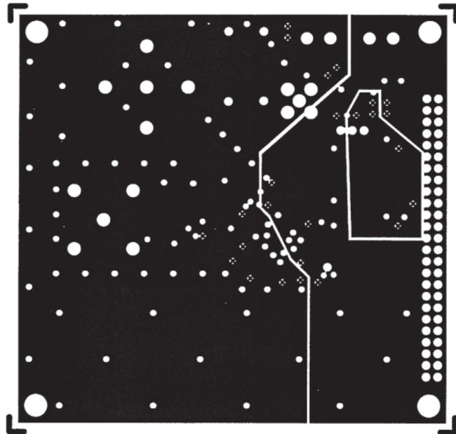
Figure 19. AD6644ST/PCB "Split" Power Layer – Layers 3 and 4 (Negative)
