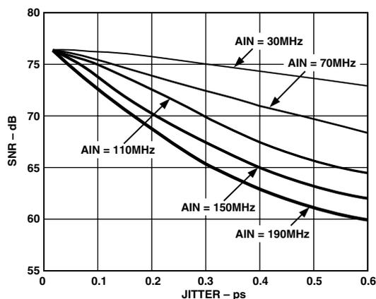
Figure 12. SNR vs. Jitter
