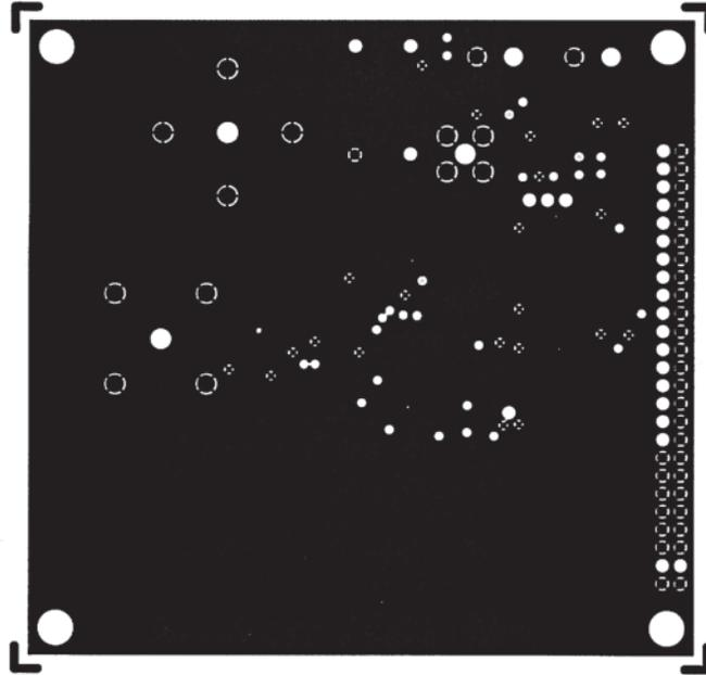
Figure 18. AD6644ST/PCB Ground Layer – Layers 2 and 5 (Negative)
