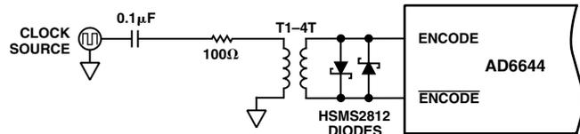
Figure 8. Crystal Clock Oscillator – Differential Encode
