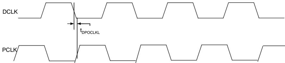
Figure 7. PCLK to DCLK Switching Characteristics Divide by 1
