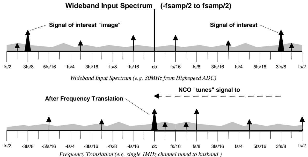
**Figure 28. AD6652 Frequency Translation of Wideband Input Spectrum**
