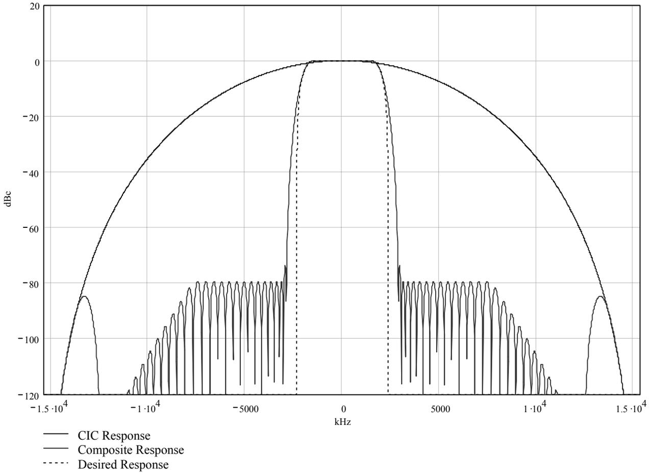
**Figure 29. Composite Filter Response of rCIC2, CIC5, and RCF**
