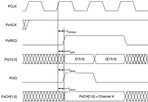
Figure 35. Channel mode interleaved format.
