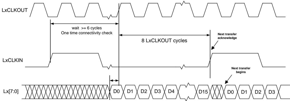
Figure 16. LxCLKIN to LxCLKOUT Data Switching Characteristics
