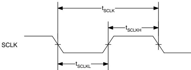
Figure 43. SCLK Timing Requirements
