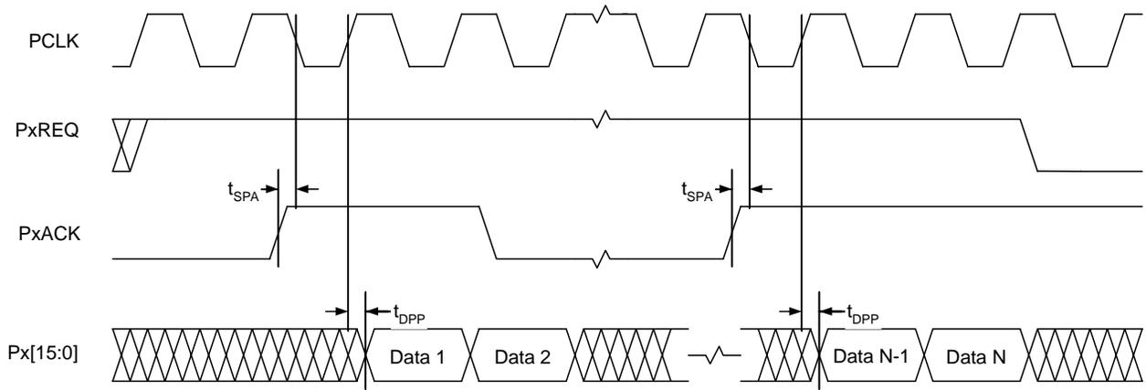
Figure 10. Master Mode PxACK to PCLK Switching Characteristics
