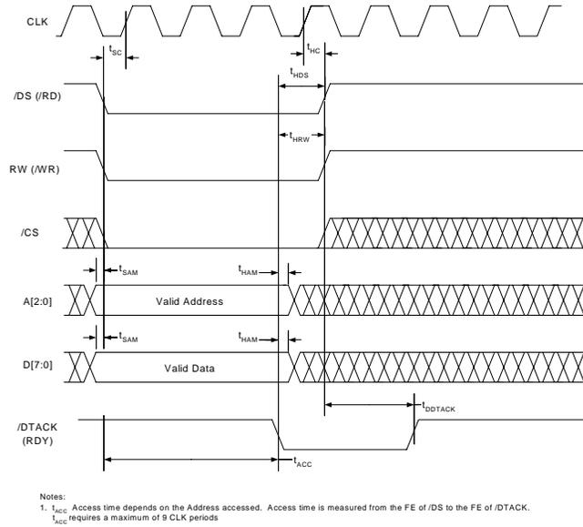
Figure 20. MNM Microport Write Timing Requirements.
