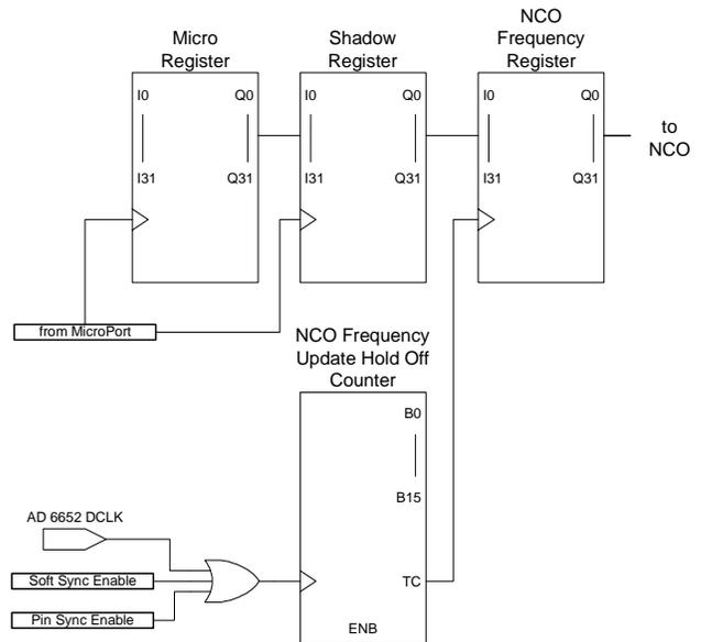
Figure 33. NCO Shadow Register and Hold Off Counter
