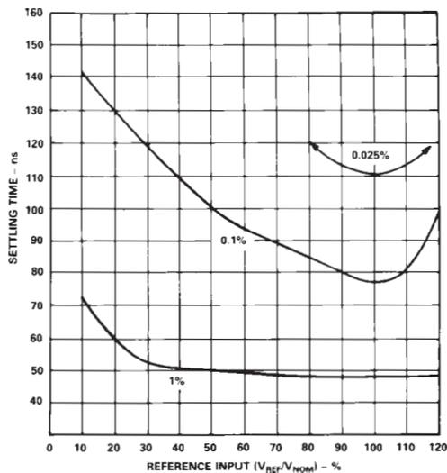
Figure 24. Digital Settling Time vs. Reference Level
