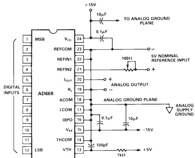
Figure 7. 5 V REF<sub>IN</sub>/1 V Unbuffered Unipolar Output
