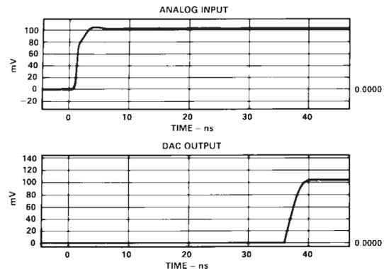
Figure 26. Undervoltage Recovery
