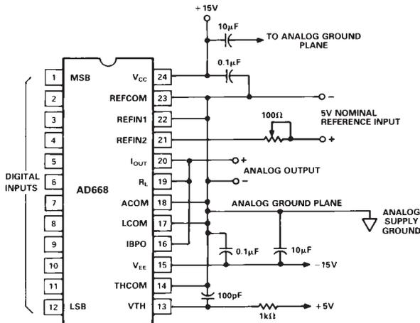
Figure 9. 5 V REFIN±1 V Unbuffered Bipolar Output
