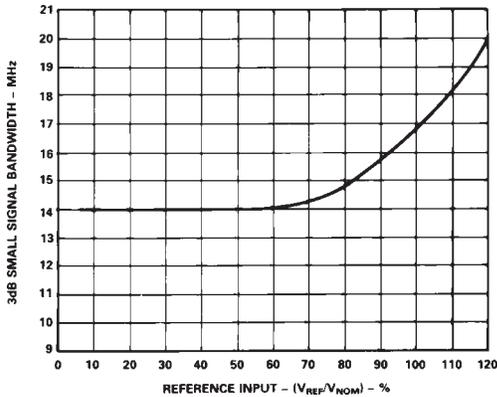
Figure 18. Small Signal Bandwidth vs. DC Reference Level
