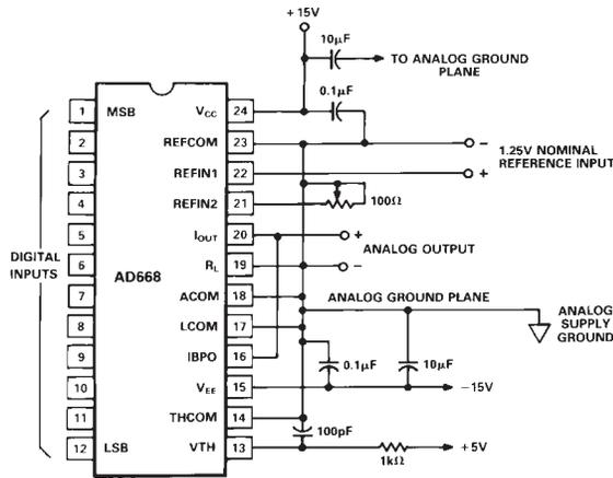
Figure 8. 1.25 V REFIN±500 mV Unbuffered Bipolar Output
