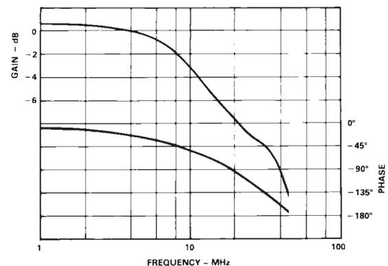
Figure 17. Large Signal Gain and Phase Response
