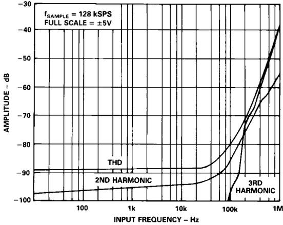
Figure 13. Harmonic Distortion vs. Input Frequency (-0.5 dB Input)
