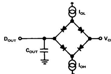
Figure 4. Load Circuit for Bus Timing Specifications
