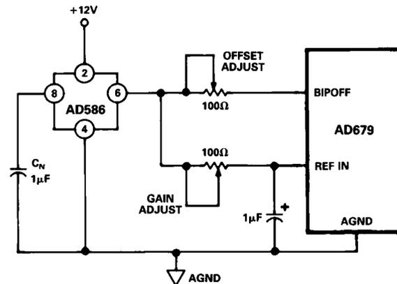
Figure 7. Bipolar Input with Gain and Offset Trims
