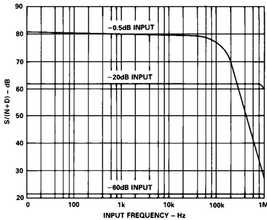
Figure 15.  $S/(N+D)$  vs. Input Frequency and Amplitude
