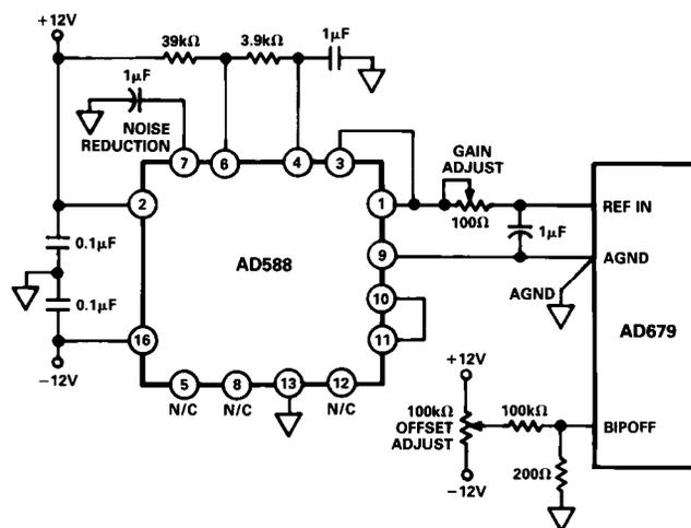
Figure 8. Unipolar Input with Gain and Offset Trims
