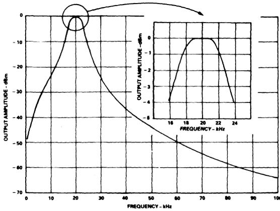
Figure 20. Output Amplitude vs. Frequency of 1/3 Octave Filter
