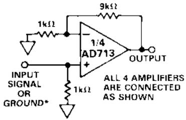
\*THE SIGNAL INPUT (1kHz SINWAVE, 2V p-p) IS APPLIED TO ONE AMPLIFIER AT A TIME. THE OUTPUTS OF THE OTHER THREE AMPLIFIERS ARE THEN MEASURED FOR CROSSTALK.
