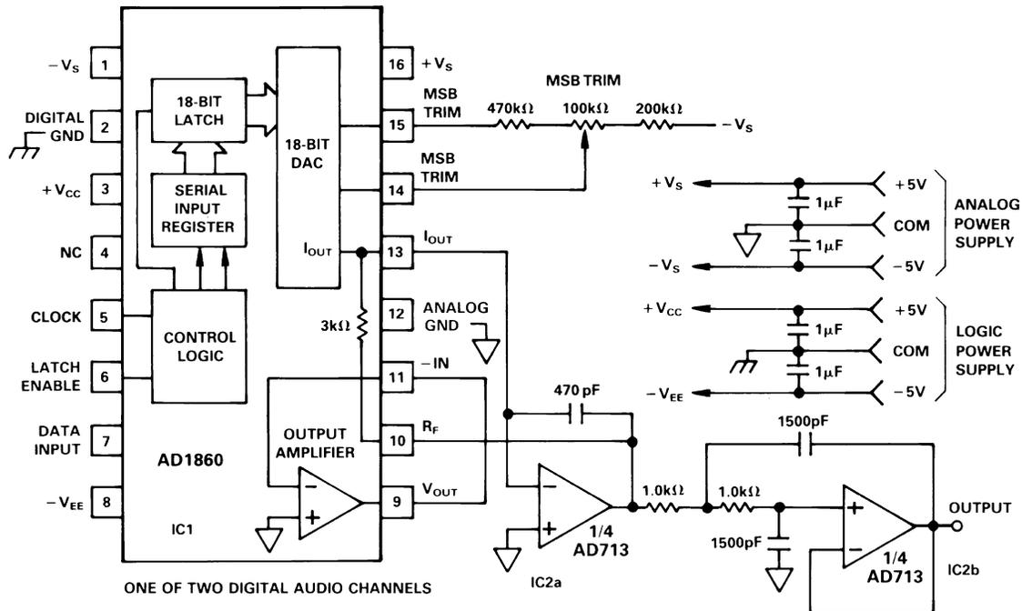
Figure 9. A D/A Converter Circuit for Digital Audio
