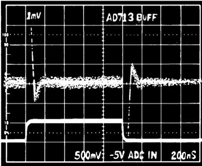
Figure 13. Buffer Recovery Time Sink Current = 1 mA
