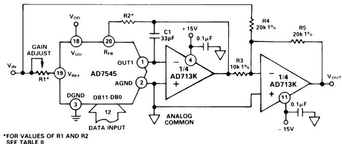
Figure 17. Bipolar Operation
