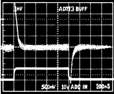
Figure 12. Buffer Recovery Time Source Current = 2 mA
