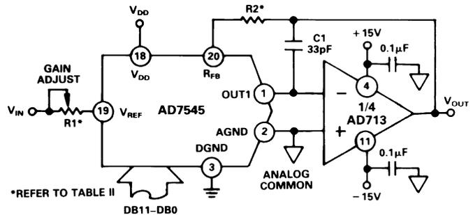
Figure 16. Unipolar Binary Operation
