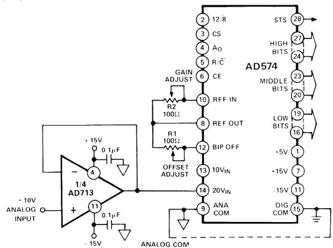
Figure 11. The AD713 as an ADC Buffer
