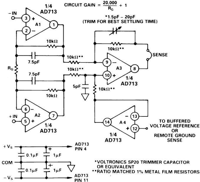
Figure 5. A High Speed Instrumentation Amplifier Circuit
