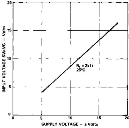
TPC 1. Input Voltage Swing vs. Supply Voltage
