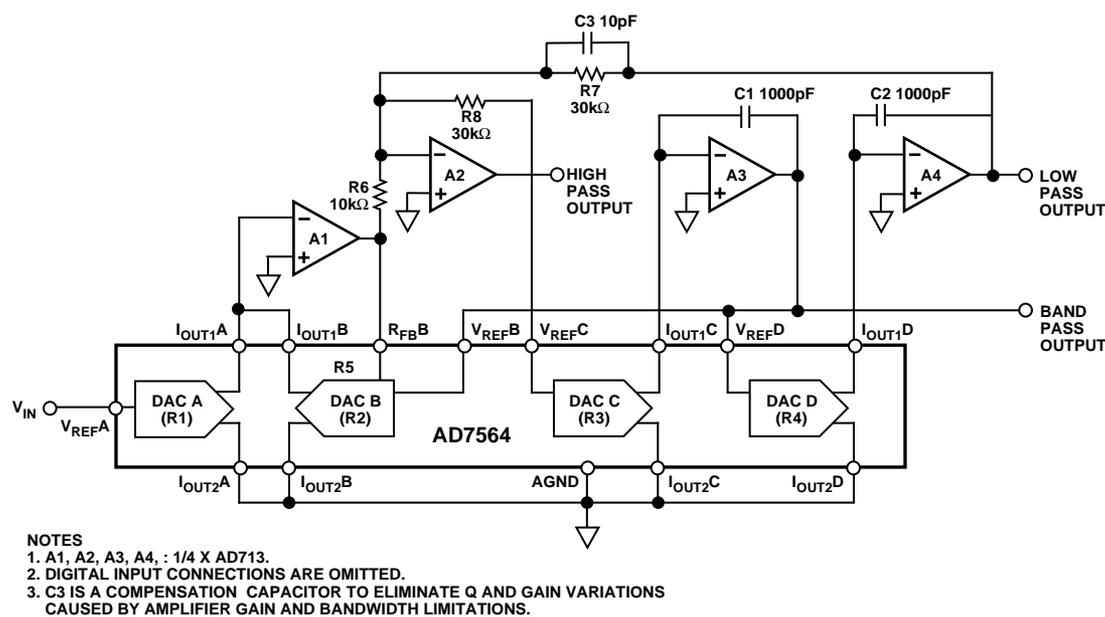
Figure 25. Programmable 2nd Order State Variable Filter
