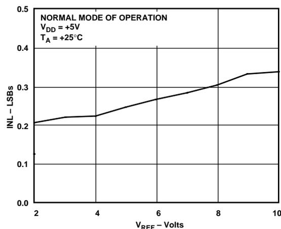
Figure 6. Integral Nonlinearity Error vs.  $V_{REF}$  (Normal Mode)
