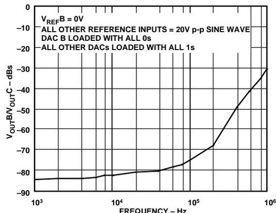
Figure 7. Channel-to-Channel Isolation (1 DAC to All Other DACs)
