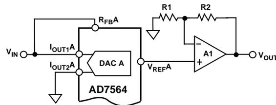
Figure 20. Single Supply Voltage Switching Mode Operation
