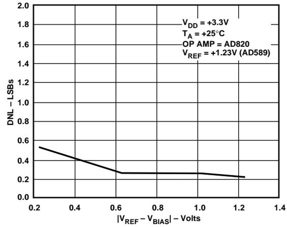
Figure 12. Differential Nonlinearity Error vs.  $V_{REF}$  (Biased Mode)
