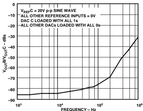
Figure 4. Channel-to-Channel Isolation (1 DAC to 1 DAC)
