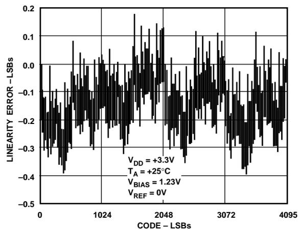
Figure 11. All Codes Linearity Plot (Biased Mode)
