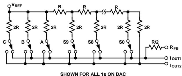
Figure 15. Simplified D/A Circuit Diagram
