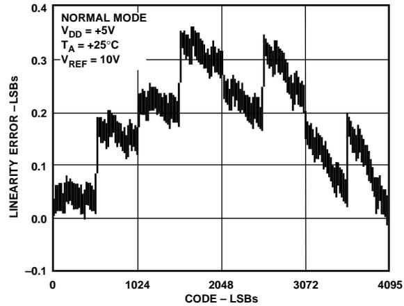
Figure 14. All Codes Linearity Plot (Normal Mode)
