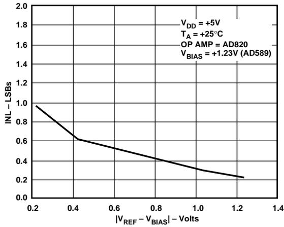
Figure 10. Integral Nonlinearity Error vs.  $V_{REF}$  (Biased Mode)
