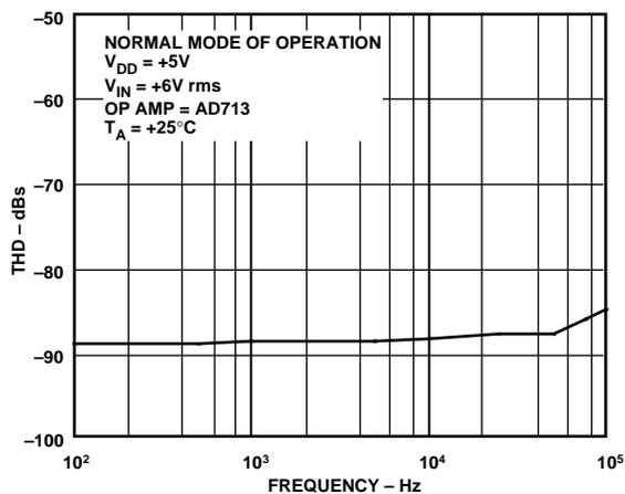
Figure 5. Total Harmonic Distortion vs. Frequency (Normal Mode)
