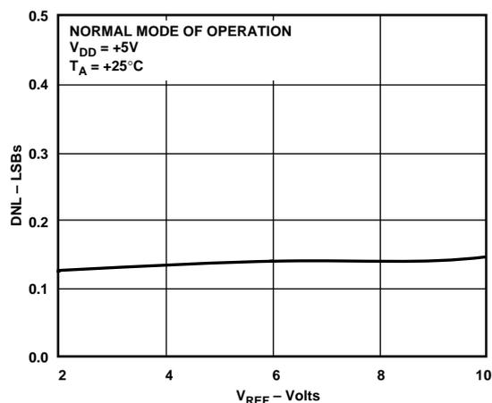
Figure 3. Differential Nonlinearity Error vs.  $V_{REF}$  (Normal Mode)
