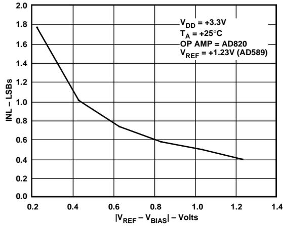
Figure 9. Integral Nonlinearity Error vs.  $V_{REF}$  (Biased Mode)
