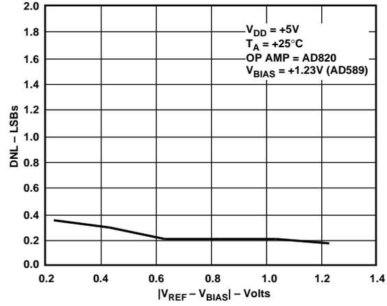
Figure 13. Differential Nonlinearity Error vs.  $V_{REF}$  (Biased Mode)
