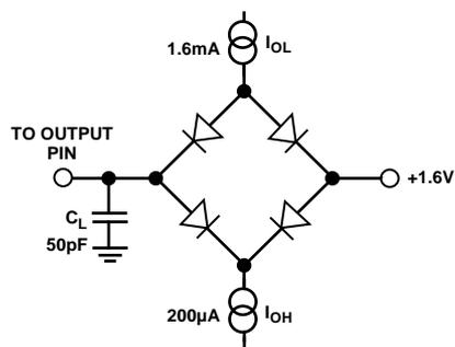
Figure 2. Load Circuit for Digital Output Timing Specifications
