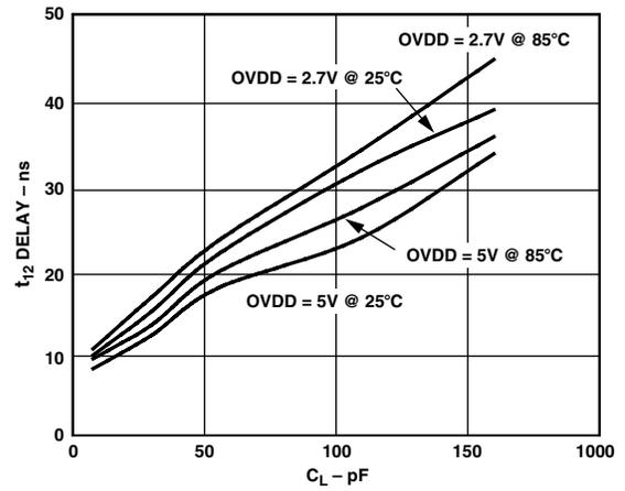
TPC 11. Typical Delay vs. Load Capacitance  $C_L$
