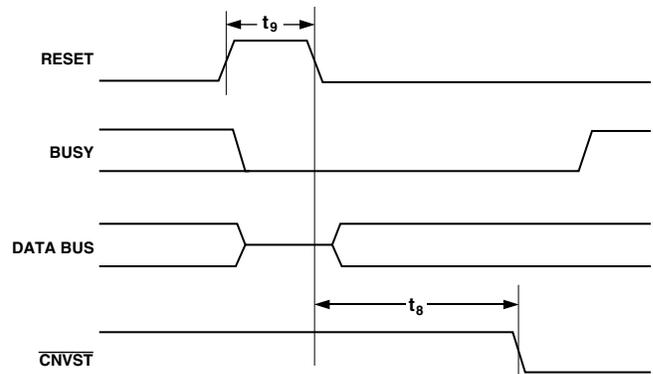
Figure 9. Reset Timing
