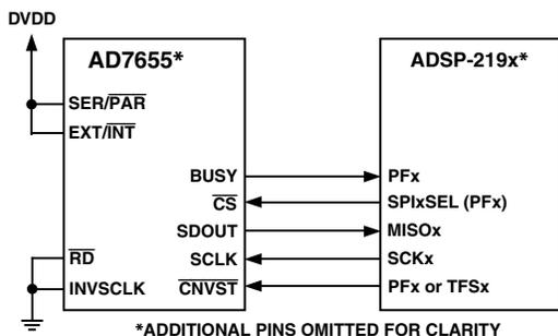
Figure 20. Interfacing the AD7655 to SPI Interface
