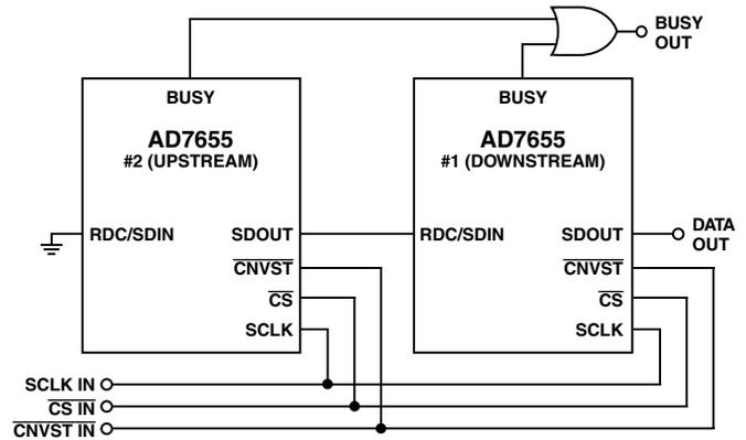
Figure 19. Two AD7655s in a Daisy-Chain Configuration
