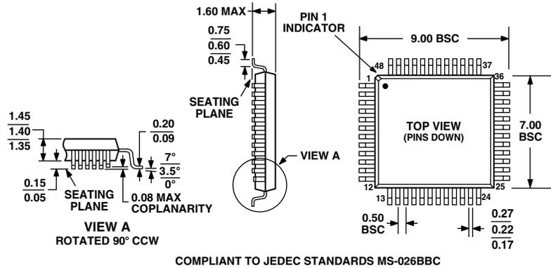
48-Lead Lead Frame Chip Scale Package [LFCSP]
