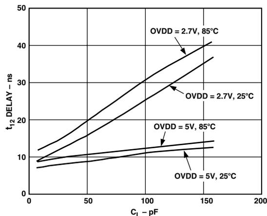
TPC 11. Typical Delay vs. Load Capacitance  $C_L$
