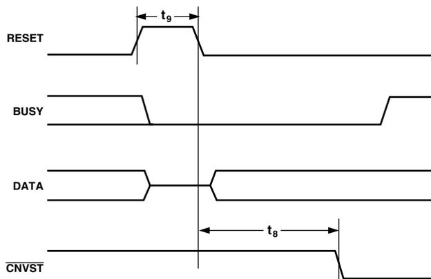
Figure 12. RESET Timing
