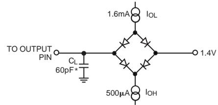
\*IN SERIAL INTERFACE MODES, THE SYNC, SCLK, AND SDOUT TIMINGS ARE DEFINED WITH A MAXIMUM LOAD CL OF 10pF; OTHERWISE, THE LOAD IS 60pF MAXIMUM.
