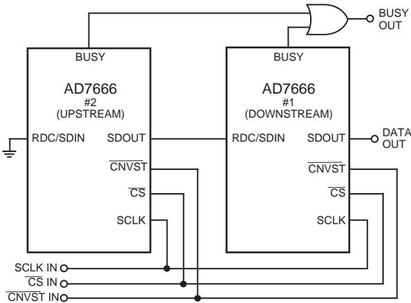
Figure 19. Two AD7666s in a “Daisy-Chain” Configuration
