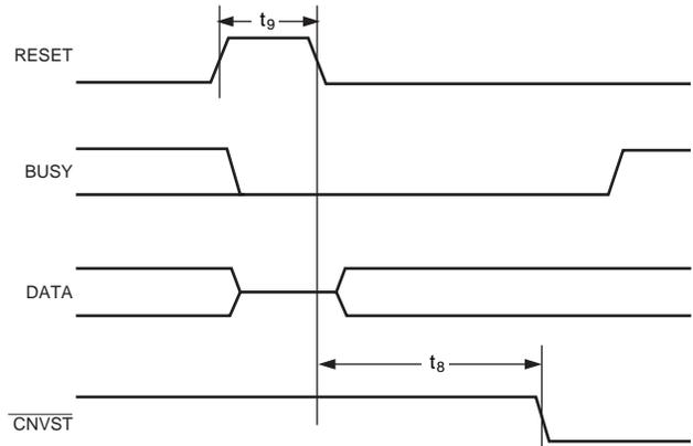
Figure 12. RESET Timing
