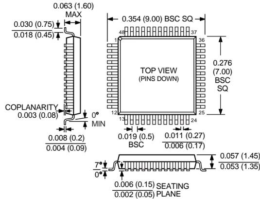
48-Lead Frame Chip Scale Package (LQFP)
