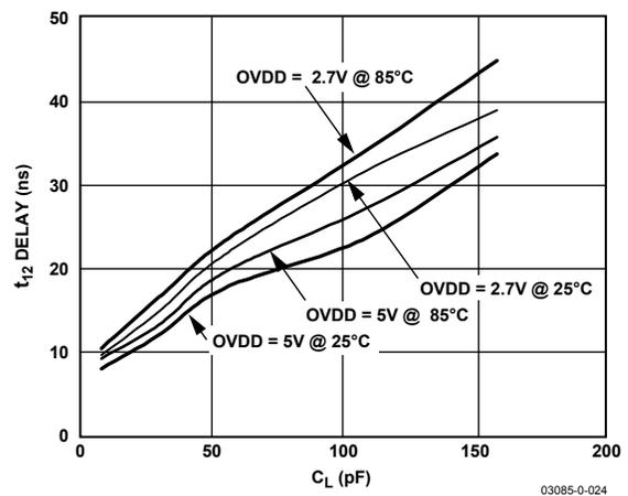
Figure 22. Typical Delay vs. Load Capacitance  $C_L$
