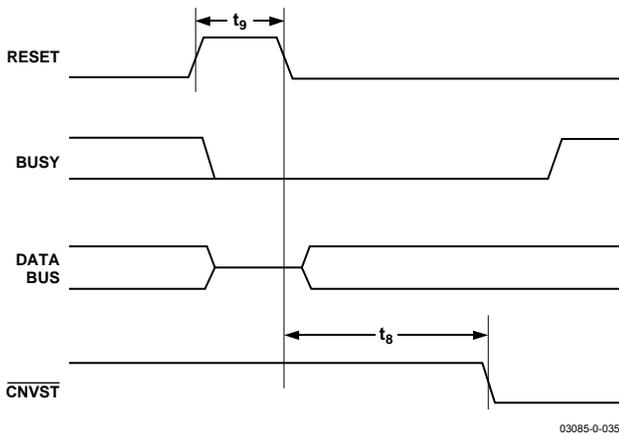
Figure 33. RESET Timing
