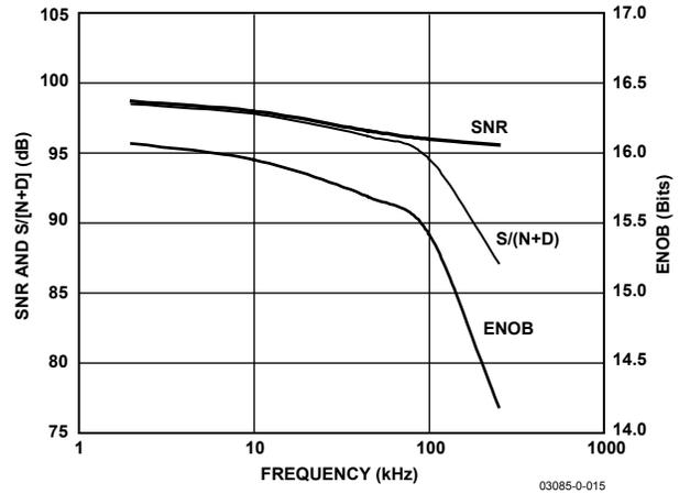
Figure 14. SNR, S/(N+D), and ENOB vs. Frequency
