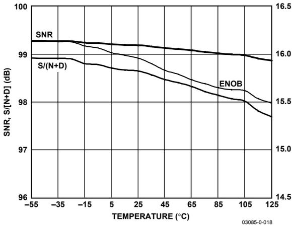
Figure 17. SNR, S/(N+D), and ENOB vs. Temperature
