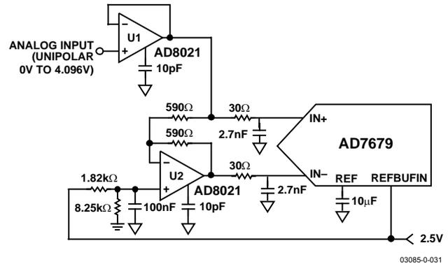
Figure 29. Single-Ended-to-Differential Driver Circuit (Internal Reference Buffer Used)
