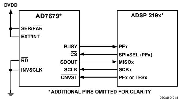
Figure 43. Interfacing the AD7679 to an SPI Interface
