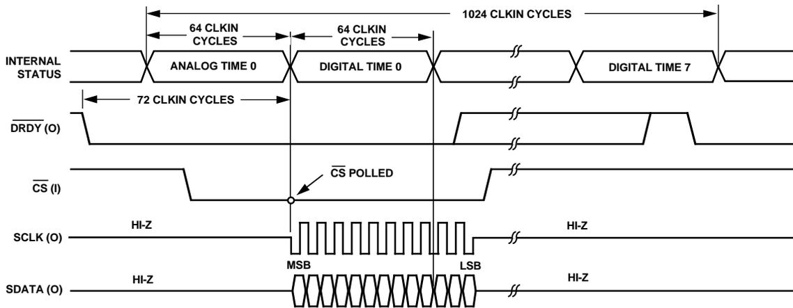
Figure 15. Timing Diagram for SSC Data Transmission Mode
