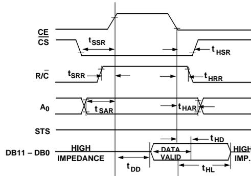
Figure 2. Read Cycle Timing
