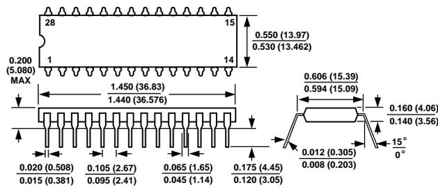
LEADS ARE SOLDER DIPPED OR TIN - PLATED ALLOY 42 OR COPPER.
