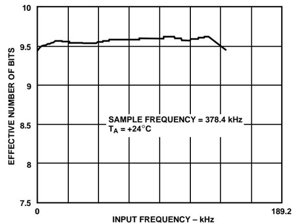
Figure 12. Effective Number of Bits vs. Frequency
