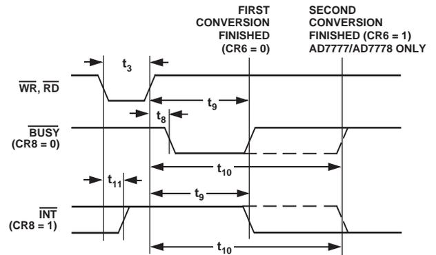
Figure 3.  $\overline{BUSY}/\overline{INT}$  Timing
