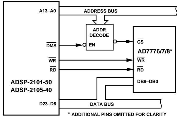
Figure 9. AD7776/AD7777/AD7778 to ADSP-2101 and ADSP-2105 Interface
