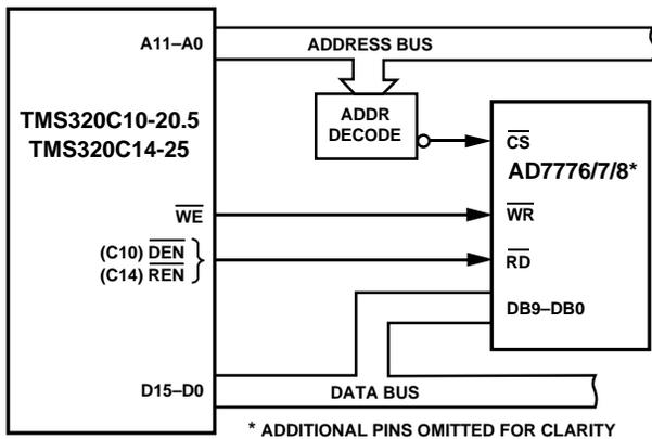
Figure 7. AD7776/AD7777/AD7778 to TMS320C10 and TMS320C14 Interface
