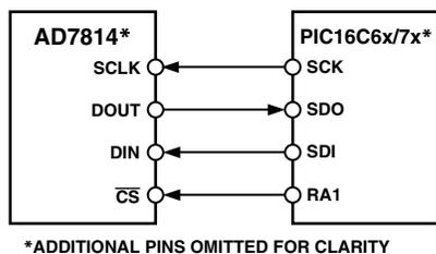
Figure 5. AD7814 to PIC16C6x/7x Interface
