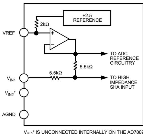
*Figure 5. AD7889-3 Analog Input Structure*
