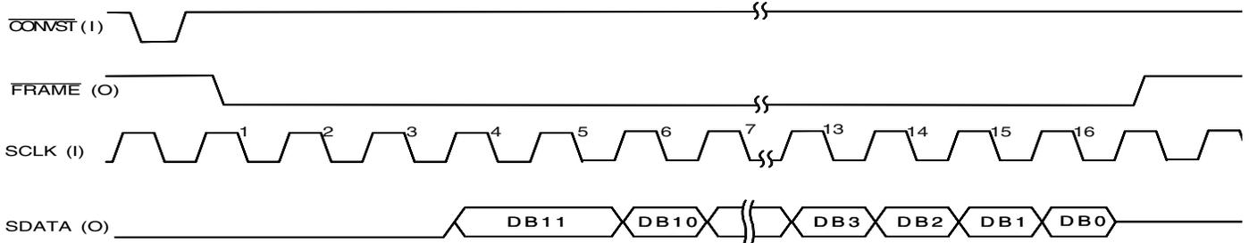
Figure 3d. Mode D Timing Diagram (IDLEHI=1)
