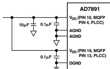
Figure 16. Recommended Decoupling Scheme for the AD7891
