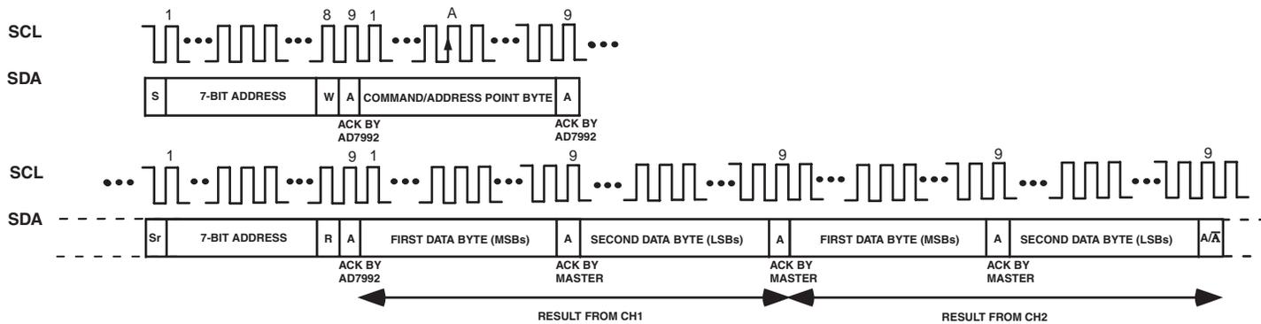
Figure 18. Mode 2 Sequence Operation
