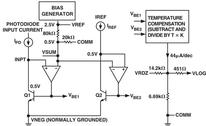
Figure 1. Simplified Schematic
