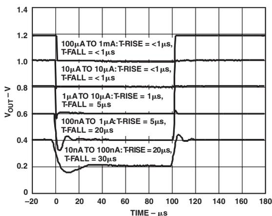
TPC 11. Pulse Response -  $I_{PD}$  to  $V_{OUT}$  ( $G = 1$ )
