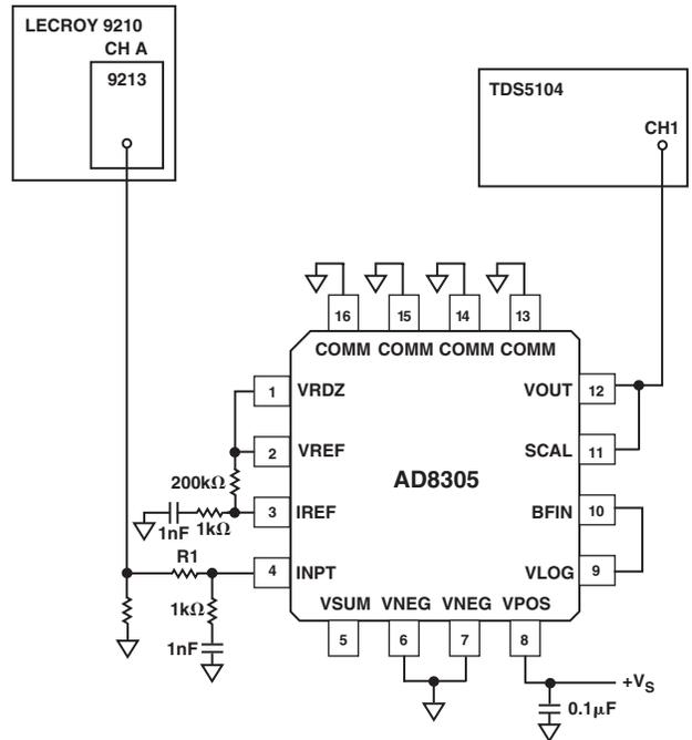
Figure 13. Configuration for Logarithmic Amplifier Pulse Response Measurement
