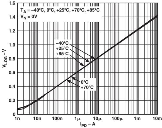
TPC 1.  $V_{LOG}$  vs.  $I_{PD}$  for Multiple Temperatures
