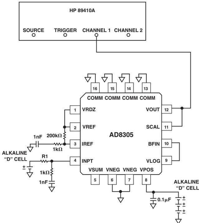
Figure 12. Configuration for Noise Spectral Density Measurement
