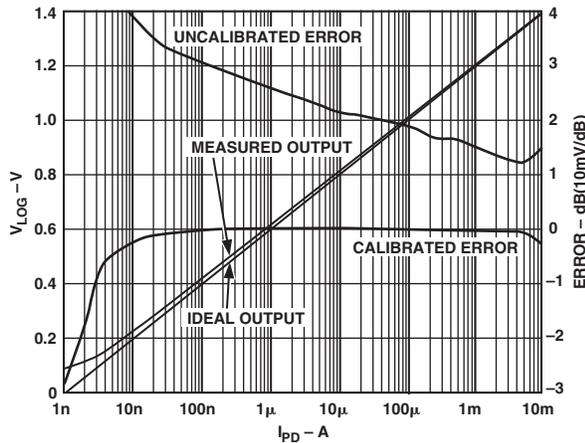
Figure 3. Using Two-Point Calibration to Increase Measurement Accuracy
