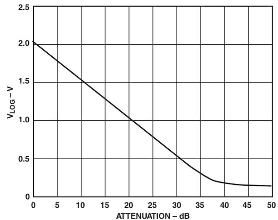
Figure 6. Example of an Absorbance Transfer Function
