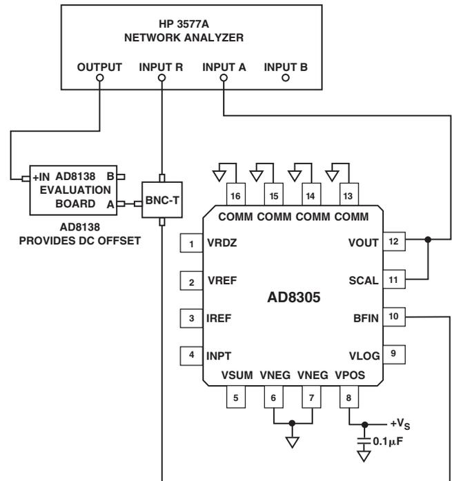
Figure 10. Configuration for Buffer Amplifier Bandwidth Measurement
