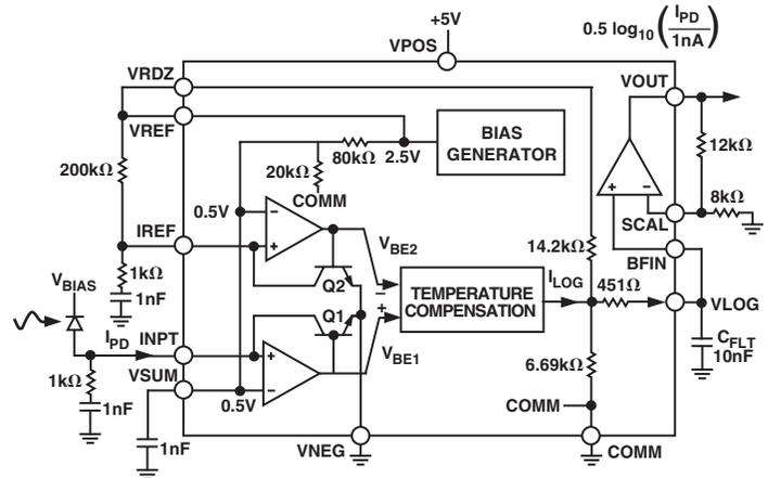
Figure 2. Basic Connections for Fixed Intercept Use
