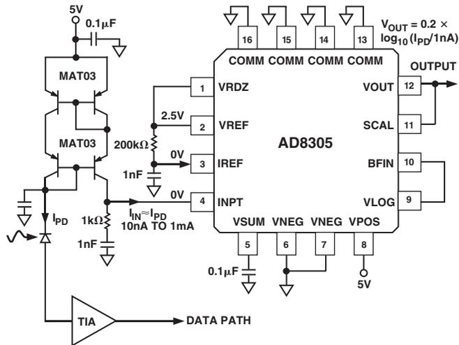
Figure 7. Wilson Current Mirror for Cathode Interfacing
