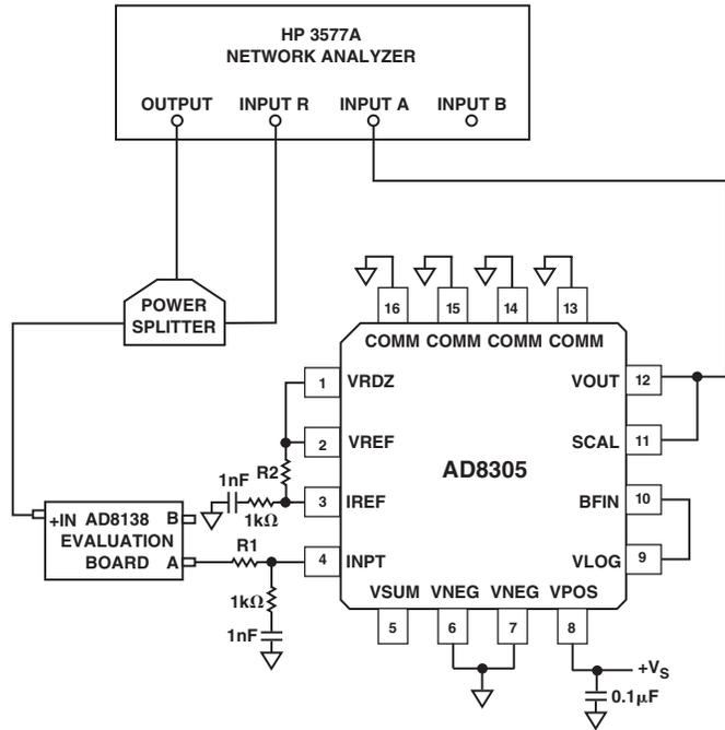
Figure 11. Configuration for Logarithmic Amplifier Bandwidth Measurement
