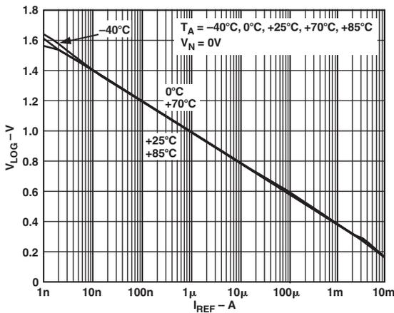
TPC 2.  $V_{LOG}$  vs.  $I_{REF}$  for Multiple Temperatures
