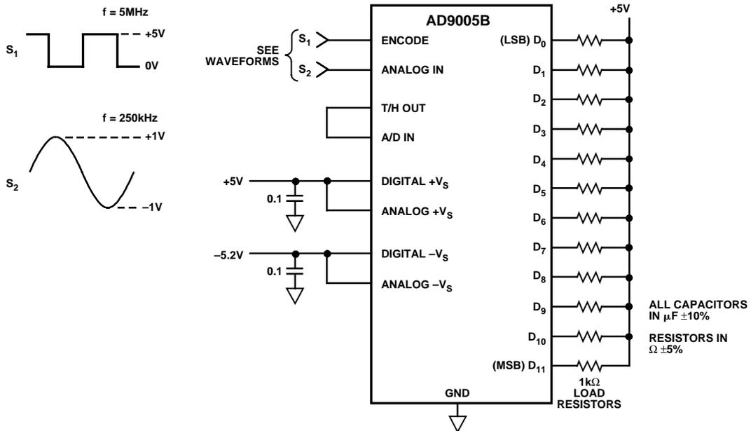
Figure 3. Burn-In Circuit
