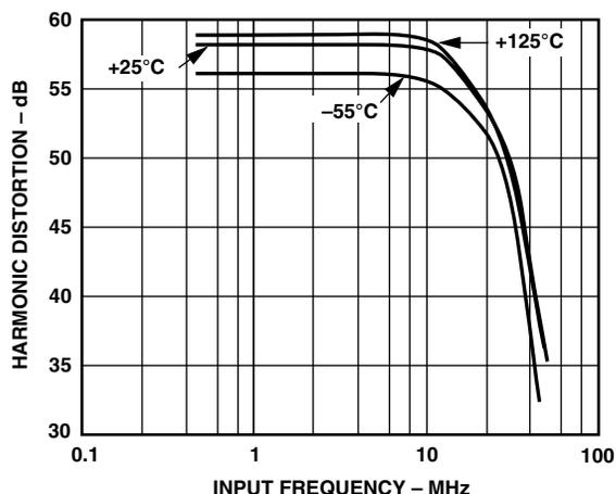
Figure 6. Harmonic Distortion vs. Analog Input Frequency
