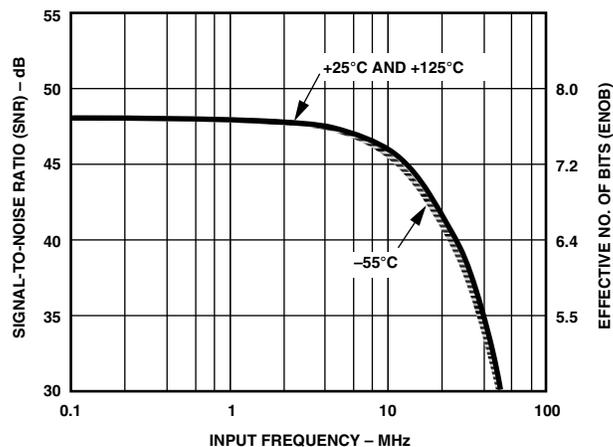
Figure 7. AD9058 Dynamic Performance vs. Analog Input Frequency
