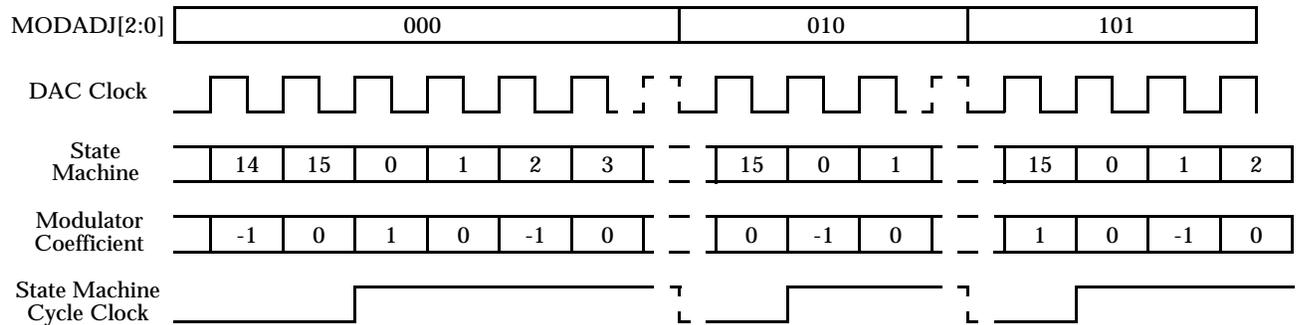
Figure 22. Local Modulator Coefficient Synchronised with Offset
