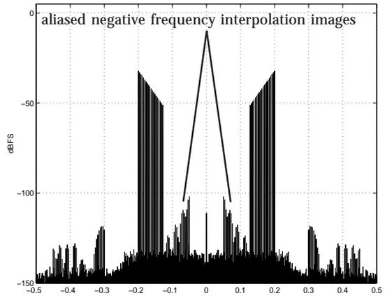
Figure 14. Negative frequency aliasing distortion
