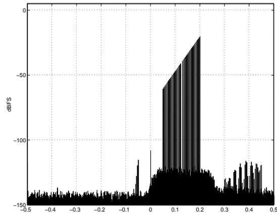
Figure 18b. Lower IF sideband rejected
