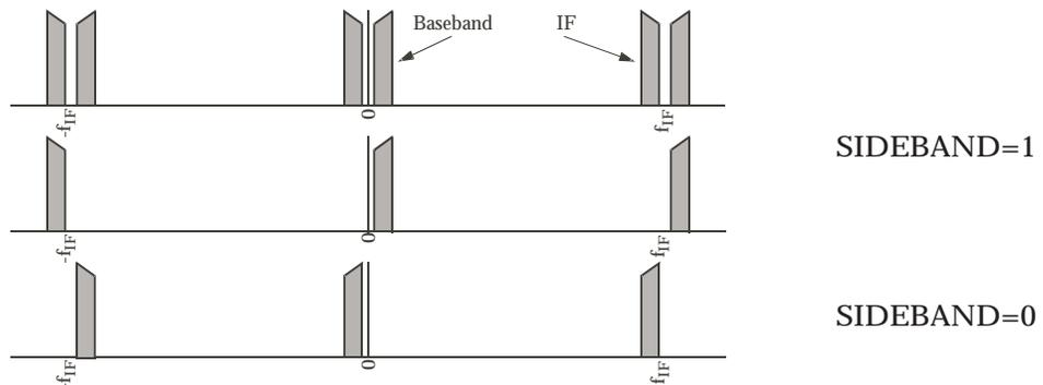
Figure 17. IF quadrature modulation of real and complex baseband signals
