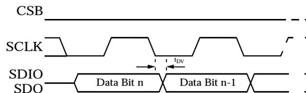
Figure 4. Timing Diagram for Register Read
