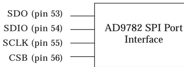
Figure 1. AD9782 SPI Port Interface
