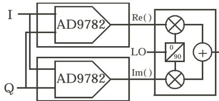
Figure 16. AD9782 Driving Quadrature Modulator
