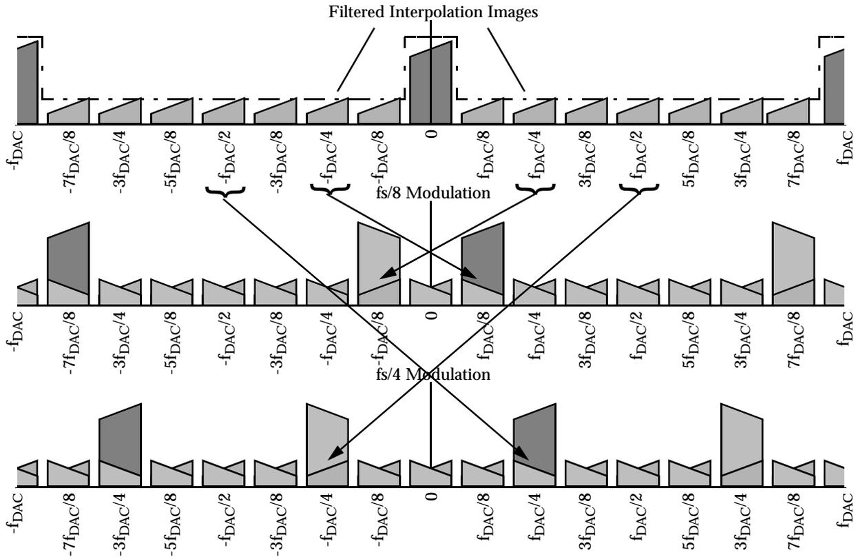
Figure 12. Complex modulation with negative frequency aliasing
