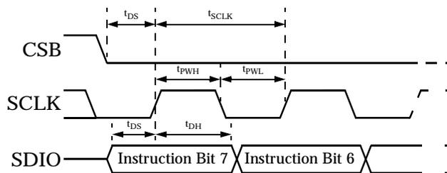
Figure 3. Timing Diagram for Register Write
