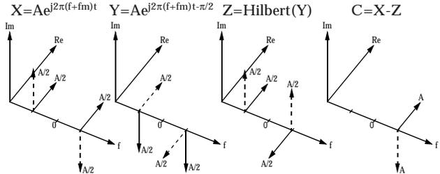
Figure 13. Negative frequency image rejection
