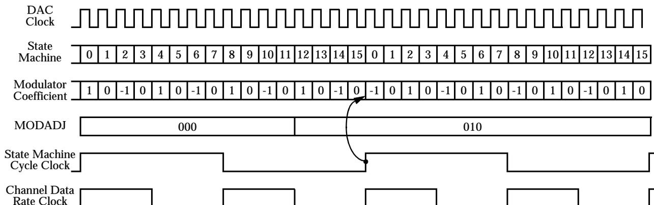
Figure 19. Synchronous Serial Modulator Phase Alignment
