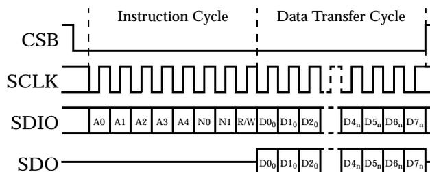
Figure 2b. Serial Register Interface Timing LSB-First
