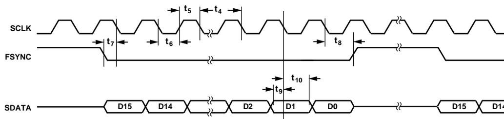
Figure 3. Serial Timing
