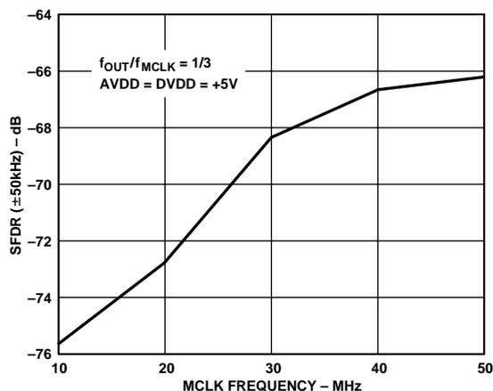
Figure 7. Narrow Band SFDR vs. MCLK Frequency
