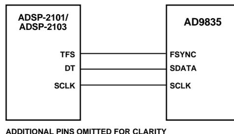
Figure 24. ADSP-2101/ADSP-2103-to-AD9835 Interface
