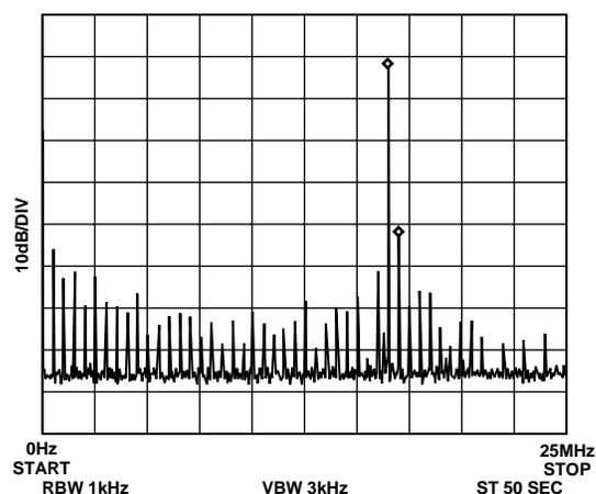
Figure 18.  $f_{MCLK} = 50$  MHz,  $f_{OUT} = 16.5$  MHz. Frequency Word = 547AE148
