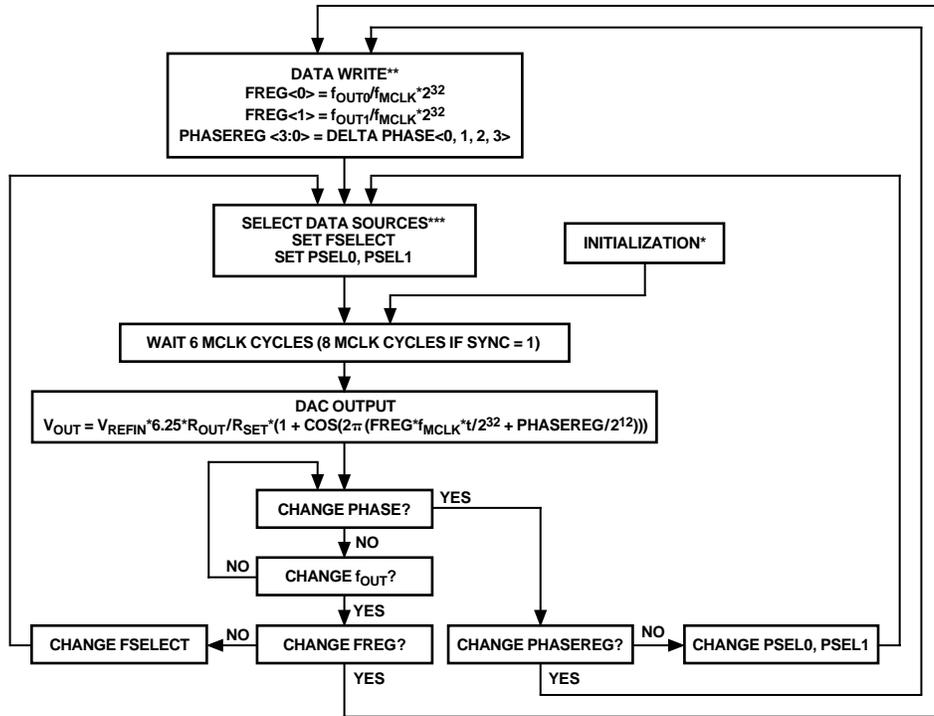
Figure 20. Flowchart for AD9835 Initialization and Operation
