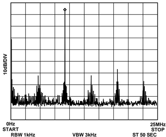
Figure 15.  $f_{MCLK} = 50$  MHz,  $f_{OUT} = 9.1$  MHz. Frequency Word = 2E978D50
