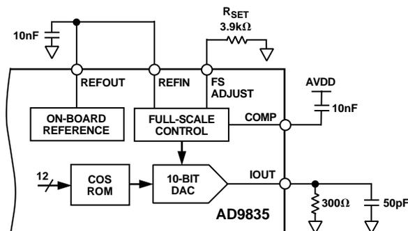
Figure 1. Test Circuit with Which Specifications Are Tested
