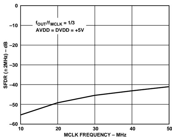
Figure 8. Wide Band SFDR vs. MCLK Frequency
