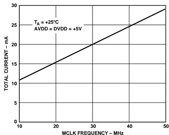
Figure 6. Typical Current Consumption vs. MCLK Frequency
