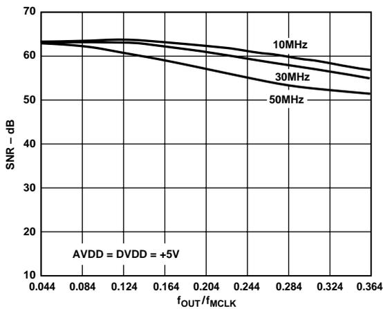
Figure 11. SNR vs.  $f_{OUT}/f_{MCLK}$  for Various MCLK Frequencies
