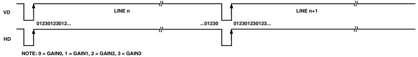
Figure 14. PxGA Mode 4 (4-Color) Frame/Line Gain Register Sequence
