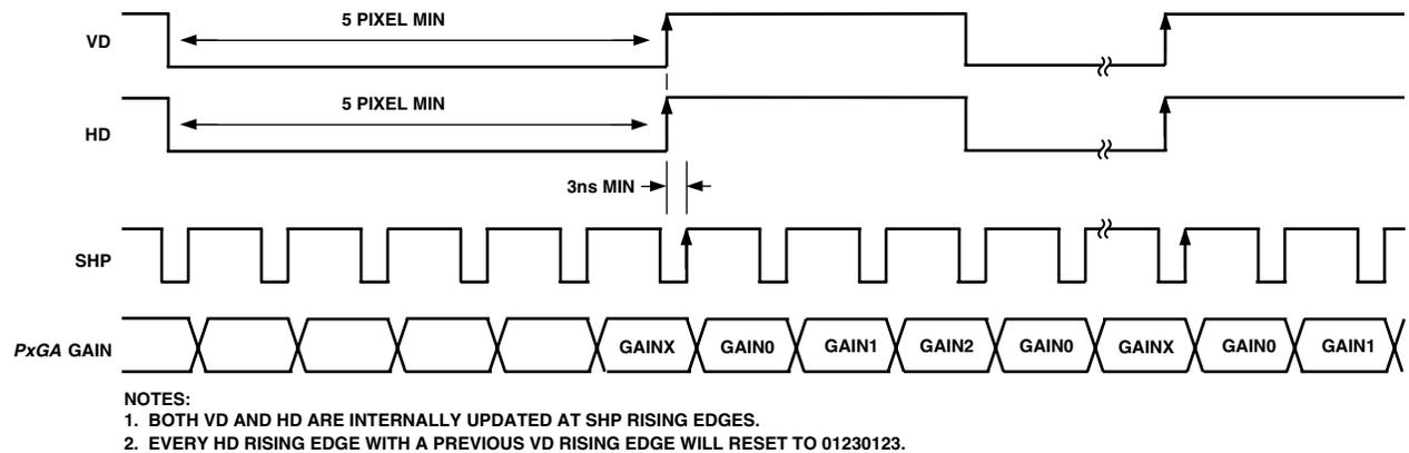
Figure 15. PxGA Mode 4 (4-Color) Detailed Timing
