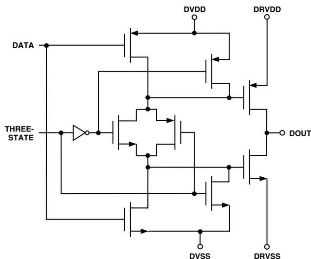
Figure 2. Data Outputs—D0–D11
