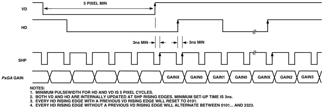
Figure 9. PxGA Mode 1 (Mosaic Separate) Detailed Timing
