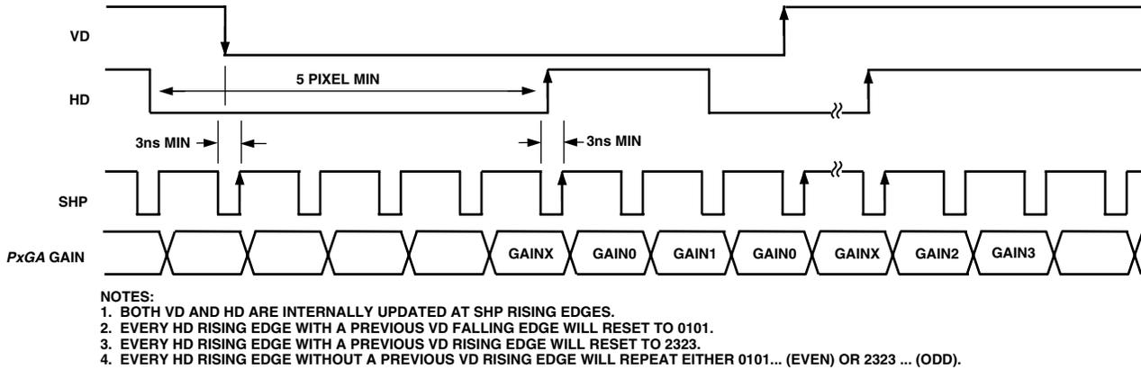
Figure 17. PxGA Mode 5 (VD Selected) Detailed Timing
