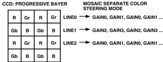
Figure 26. CCD Color Filter Example: Progressive Scan
