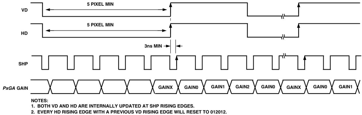
Figure 13. PxGA Mode 3 (3-Color) Detailed Timing
