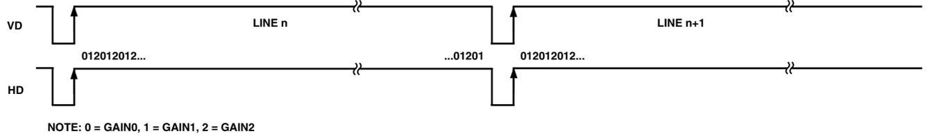
Figure 12. PxGA Mode 3 (3-Color) Frame/Line Gain Register Sequence
