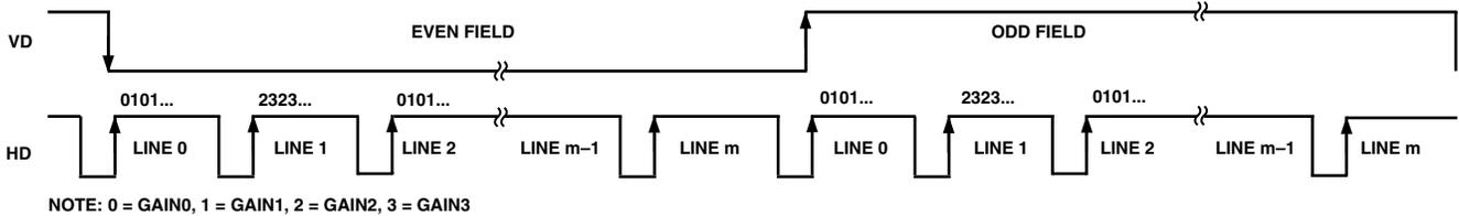
Figure 10. PxGA Mode 2 (Interlace) Frame/Line Gain Register Sequence
