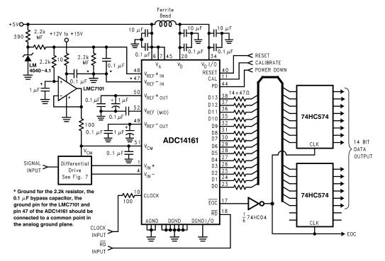
Figure 8. Simple application circuit with single-ended to differential buffer.
