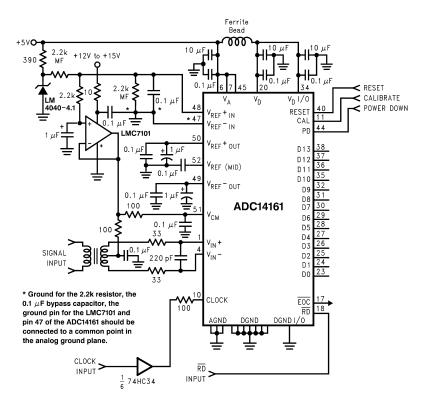
Figure 10. Driving the signal inputs with a transformer.
