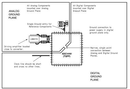
Figure 11. Example at a suitable layout.
