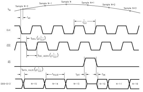
Figure 3. TIMING DIAGRAM 1. Output Timing
