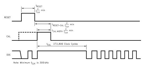
Figure 4. TIMING DIAGRAM 2. Reset and Calibration
