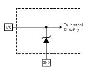
Figure 2. ESD Protection Scheme for Analog Input and Digital Output pins
