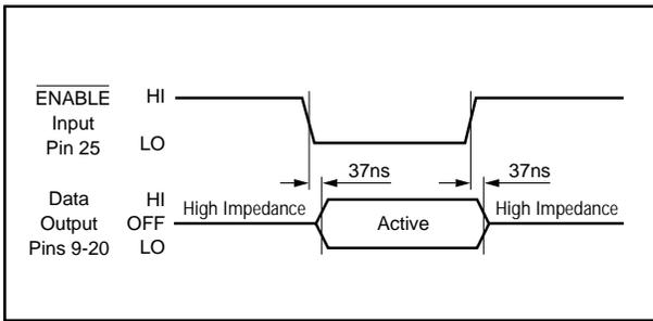
FIGURE 14. Digital Data 3-State Output.
