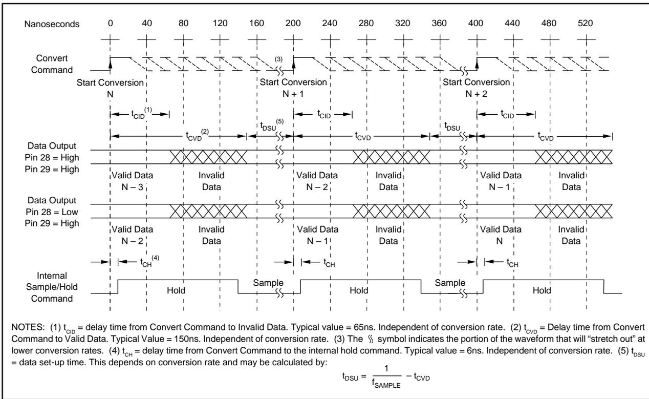
FIGURE 12. Convert Command Strobe Timing for a 5MHz Conversion Rate.
