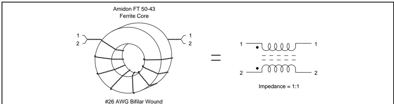
FIGURE 7. Common-Mode Choke Transformer Windings.
