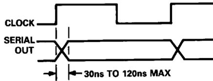
Figure 10. Clock High to Serial Out Valid
