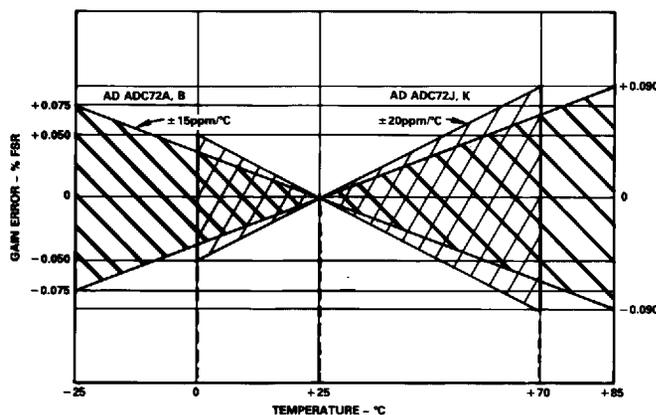
Figure 2. AD ADC72 Gain Drift Error vs. Temperature
