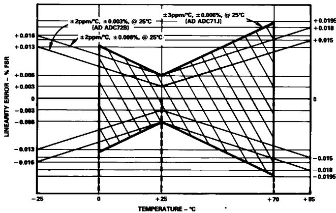
Figure 1. Linearity Error vs. Temperature
