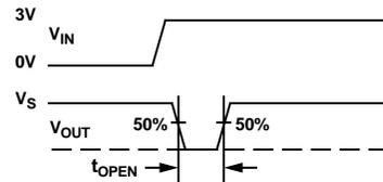
Test Circuit 5. Break-Before-Make Delay,  $t_{OPEN}$
