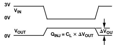
Test Circuit 6. Charge Injection
