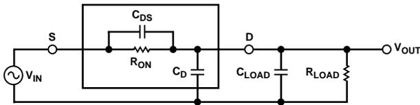
Figure 7. Switch Represented by Equivalent Parasitic Components
