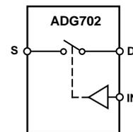
SWITCHES SHOWN FOR A LOGIC "1" INPUT
