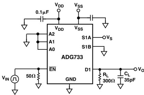
Test Circuit 5. Enable Delay,  $t_{ON}(\overline{EN})$ ,  $t_{OFF}(\overline{EN})$
