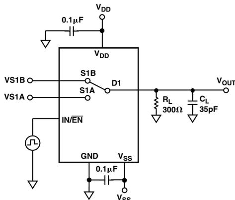
Test Circuit 4. Switching Times,  $t_{ON}$ ,  $t_{OFF}$
