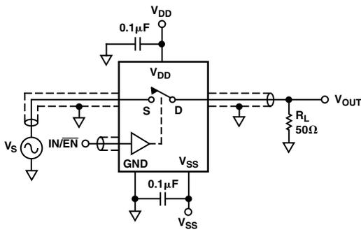
SWITCH OPEN FOR OFF ISOLATION MEASUREMENTS
