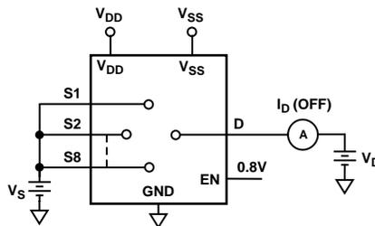
Test Circuit 3.  $I_D$  (OFF)
