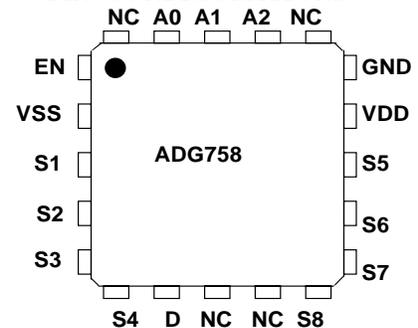
Exposed Pad tied to Substrate, V<sub>SS</sub>
