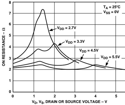
Figure 1. On Resistance as a Function of  $V_D$  ( $V_S$ ) for Single Supply
