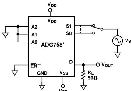
$$\text{OFF ISOLATION} = 20 \text{LOG}_{10} \frac{V_{OUT}}{V_S}$$
