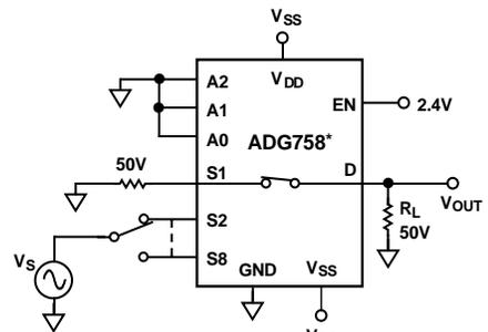
$$\text{CHANNEL-TO-CHANNEL CROSSTALK} = 20 \text{LOG}_{10} \frac{V_{OUT}}{V_S}$$
