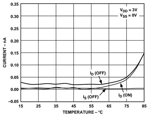
Figure 10. Leakage Currents as a Function of Temperature
