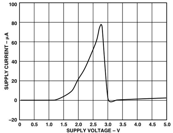
Figure 10. Standby Supply Current vs. Supply Voltage
