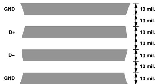
Figure 17. Arrangement of Signal Tracks
