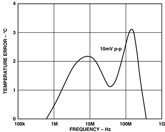
Figure 8. Temperature Error vs. Differential-Mode Noise Frequency
