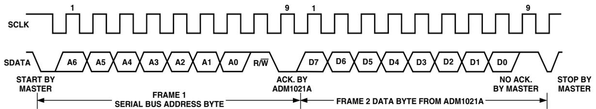
Figure 15. Reading Data from a Previously Selected Register
