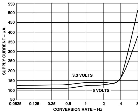
Figure 9. Operating Supply Current vs. Conversion Rate
