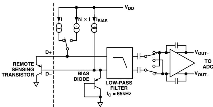
Figure 11. Signal Conditioning for External Diode Temperature Sensors
