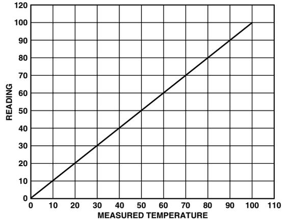
Figure 5. Pentium II® Temperature Measurement vs. ADM1025/ADM1025A Reading
