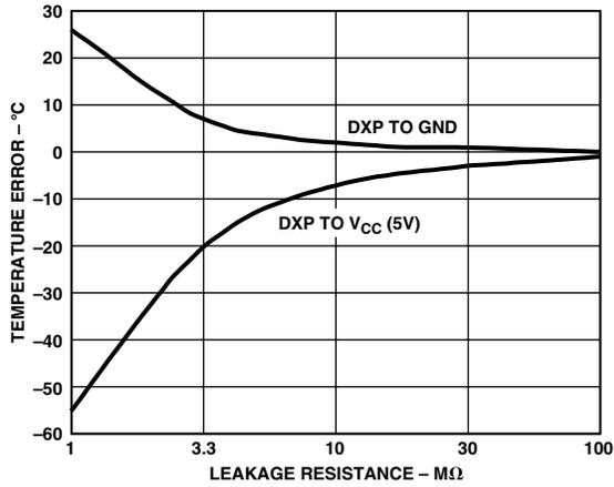
Figure 2. Temperature Error vs. PC Board Track Resistance
