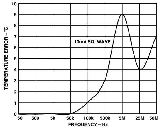
Figure 7. Temperature Error vs. Differential-Mode Noise Frequency
