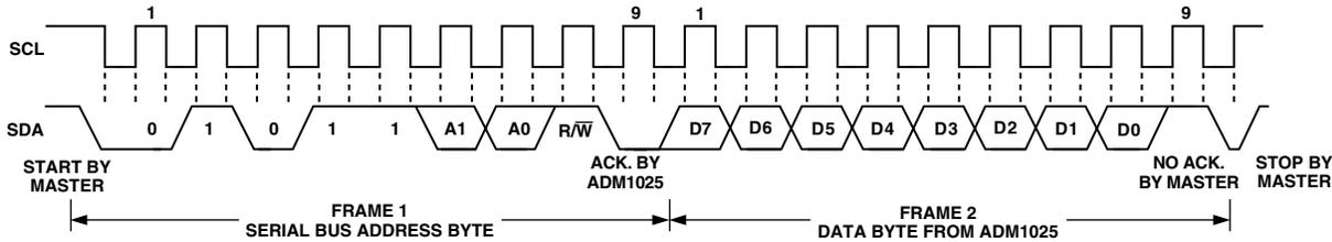
Figure 9c. Reading Data from a Previously Selected Register
