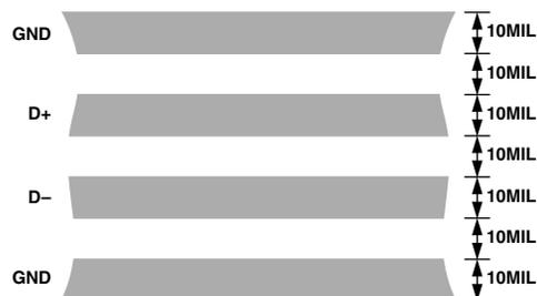
Figure 12. Arrangement of Signal Tracks
